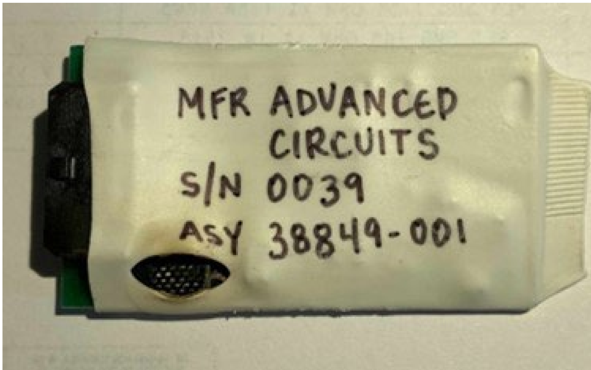
Photo 6 - Audio card exhibiting burnt resistor (Source: Cirrus).
