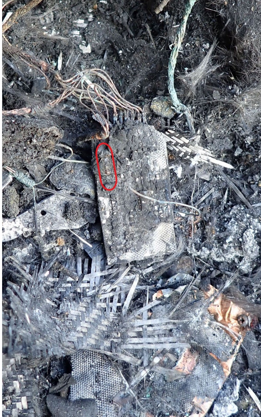
Figure 20 - Seat seven audio card with location of current-limiting resistor circled
