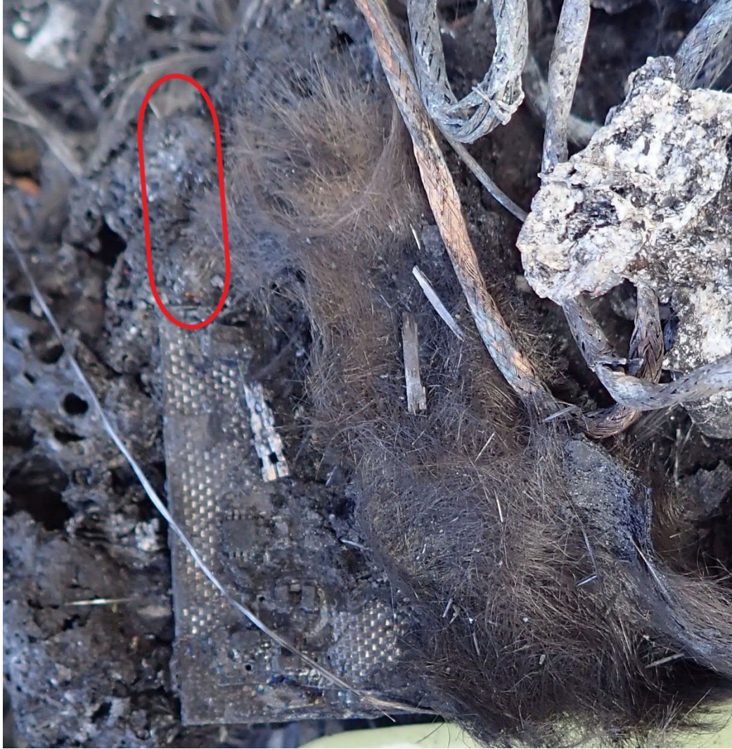
Figure 18 - Seat five audio card with location of current-limiting resistor circled
