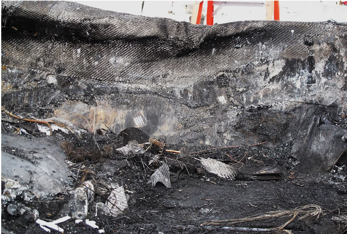
Figure 11. Damage demarcation line on right sidewall after wire bundle removal.
