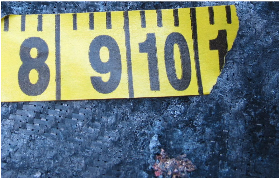
Figure 14. Copper-colored deposit with scale.
