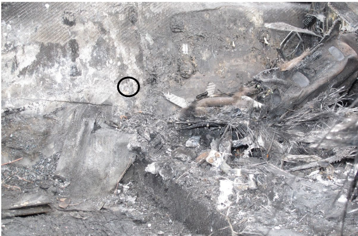
Figure 12. Close-up of demarcation line on right sidewall. Copper-colored residue (close-up shown in Figure 13) highlighted by black circle.
