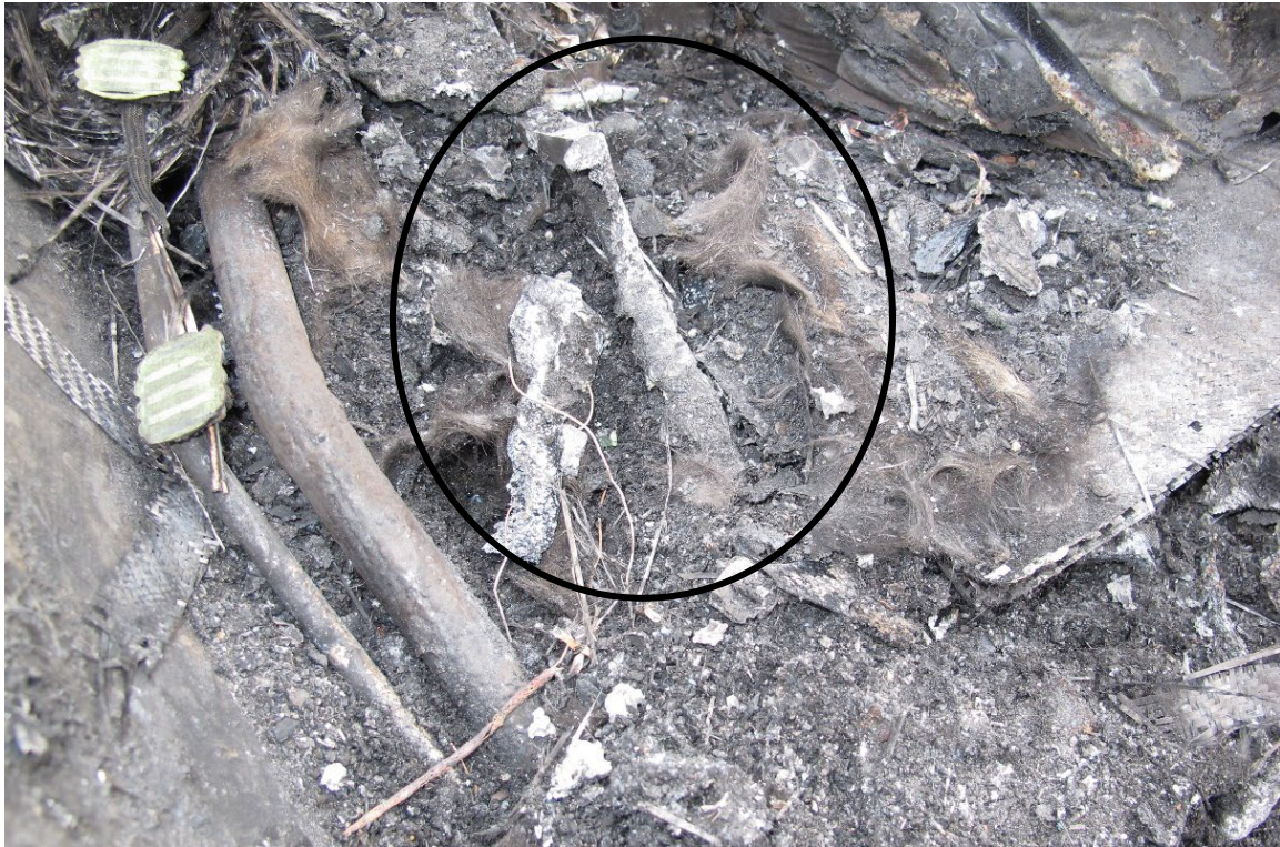
Figure 15. Area of thermal damaged seat structure (highlighted by black circle).
