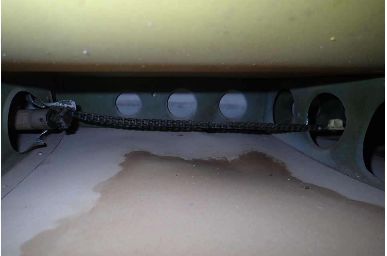
Elevator trim tab actuator, ASI-19-DH-076
