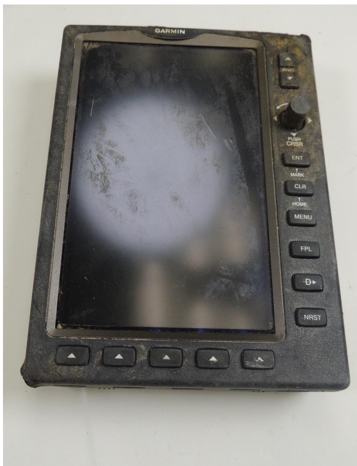
Figure 2. Photo of Garmin 695 showing minor external thermal damage and sooting.
