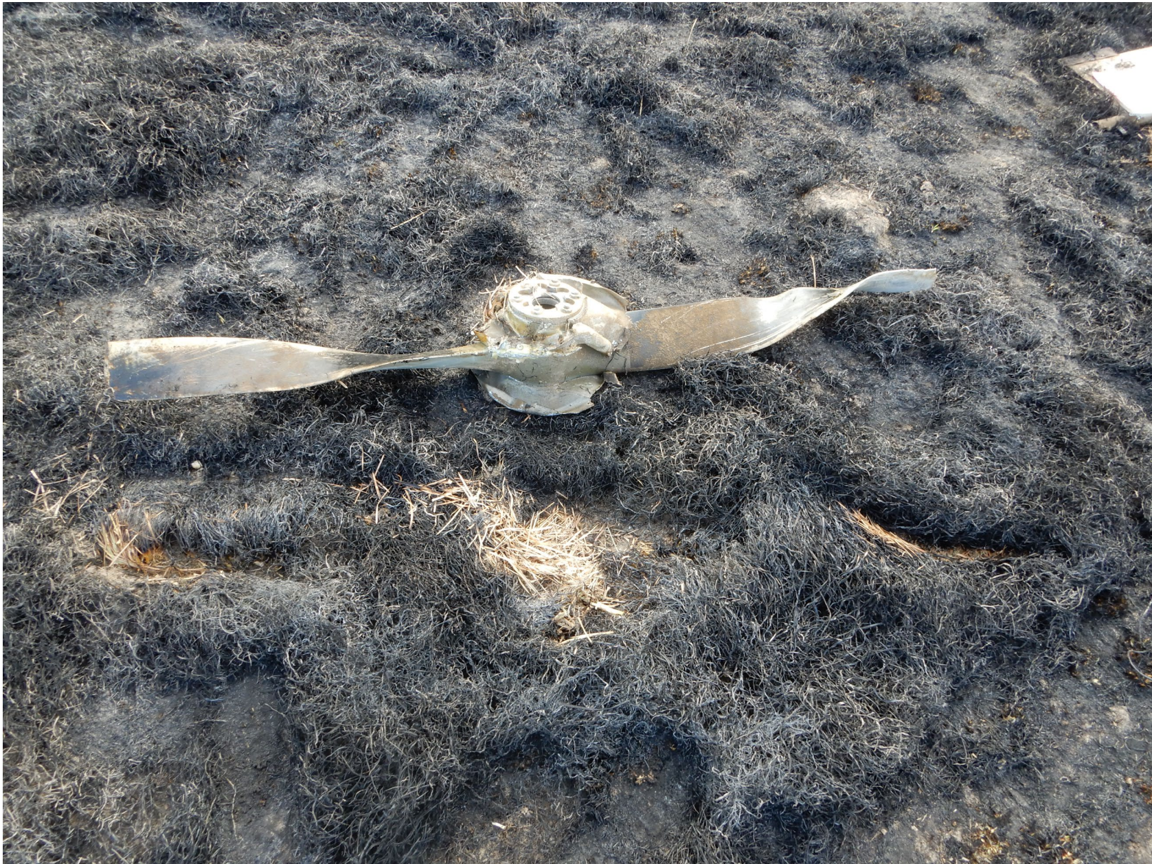
Photo 5 – Propeller Blades and Hub in Debris Field
