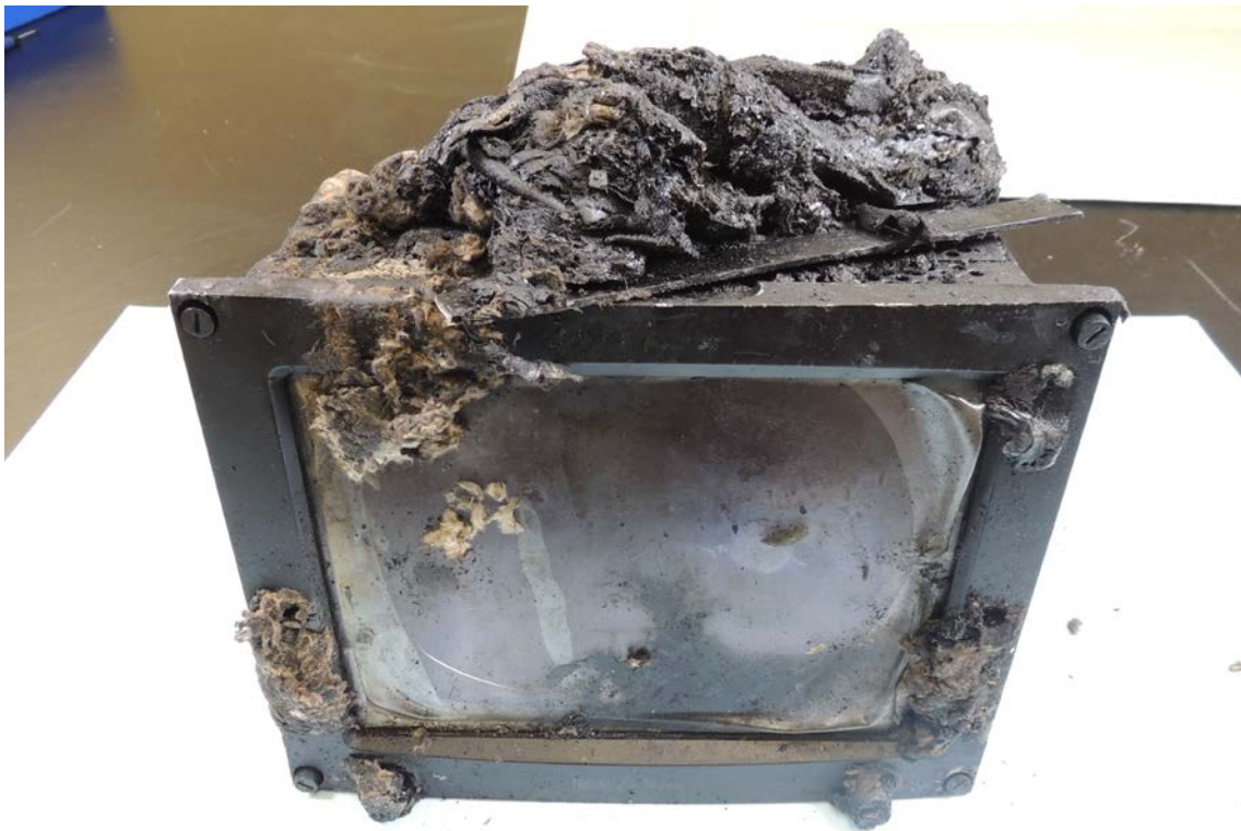
Figure 1. Photo of damaged PFD.
