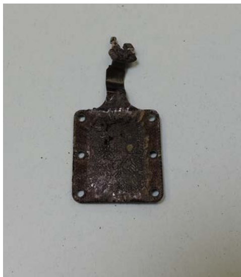
Figure 2. Photo of damaged DFC-90 memory module.
