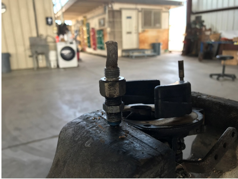
Photo 5: View of the carburetor fuel screen.
