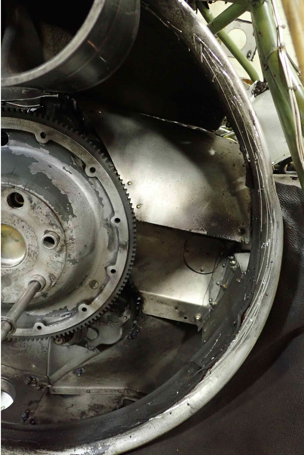
Photo 8 – Cooling Fan Shroud
