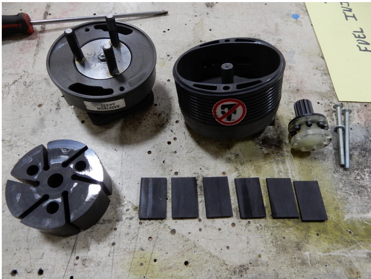
Figure 17. Vacuum pump. Photo courtesy of Continental Aerospace Technologies.
