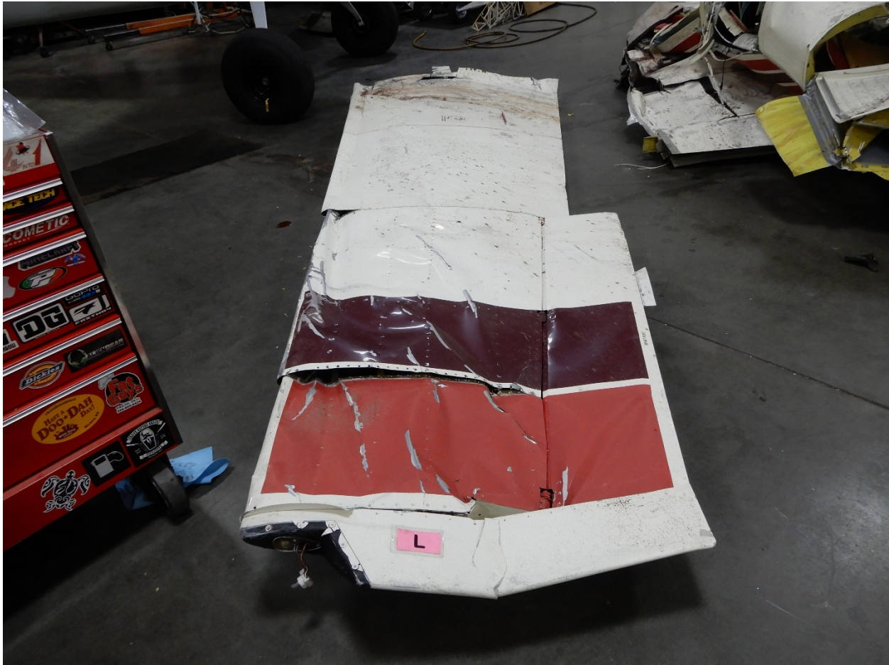
Figure 9. The left wing, top-side view, showing the aileron, and composite wing tip.
