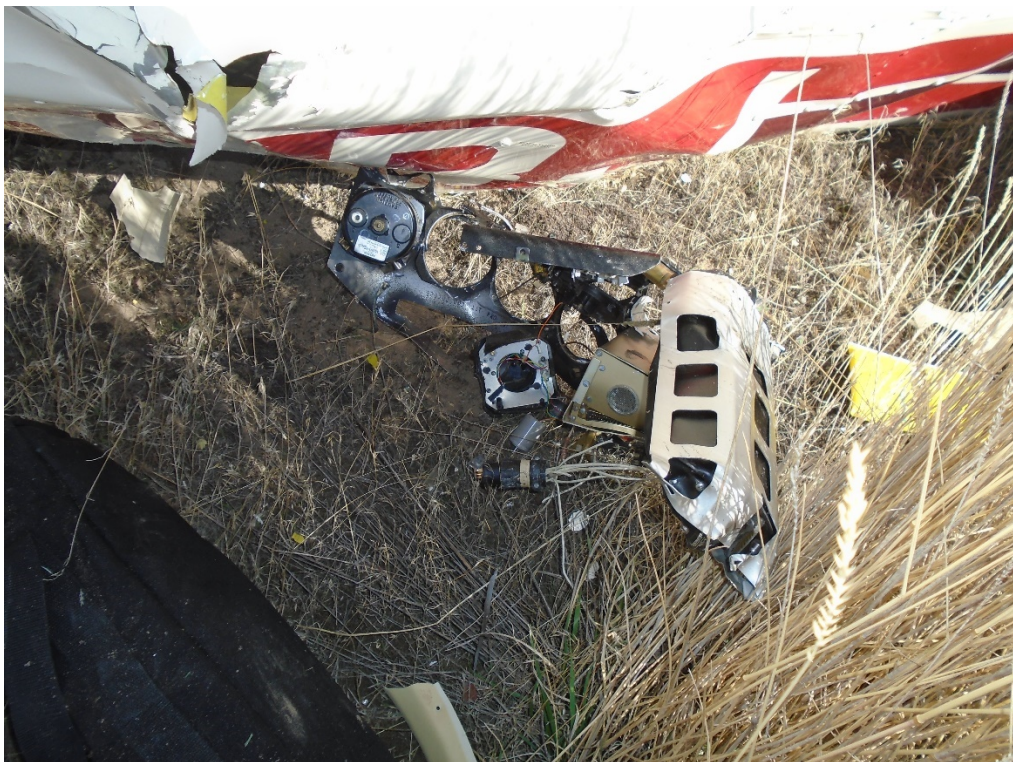
Figure 4. Instrument panel as found at accident site.
