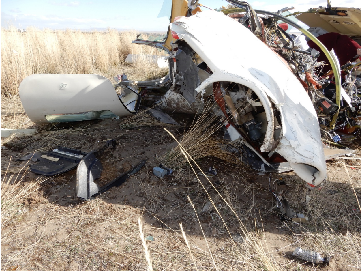
Figure 5. Front view, showing the displaced upper engine cowling.
