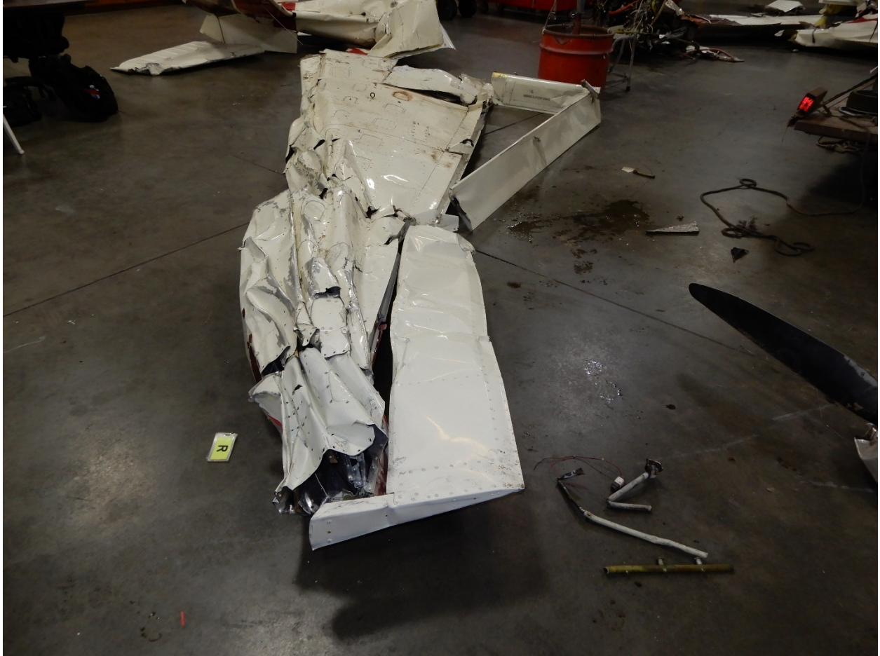
Figure 8. The right wing, underside view, showing the aileron and partially attached flap.
