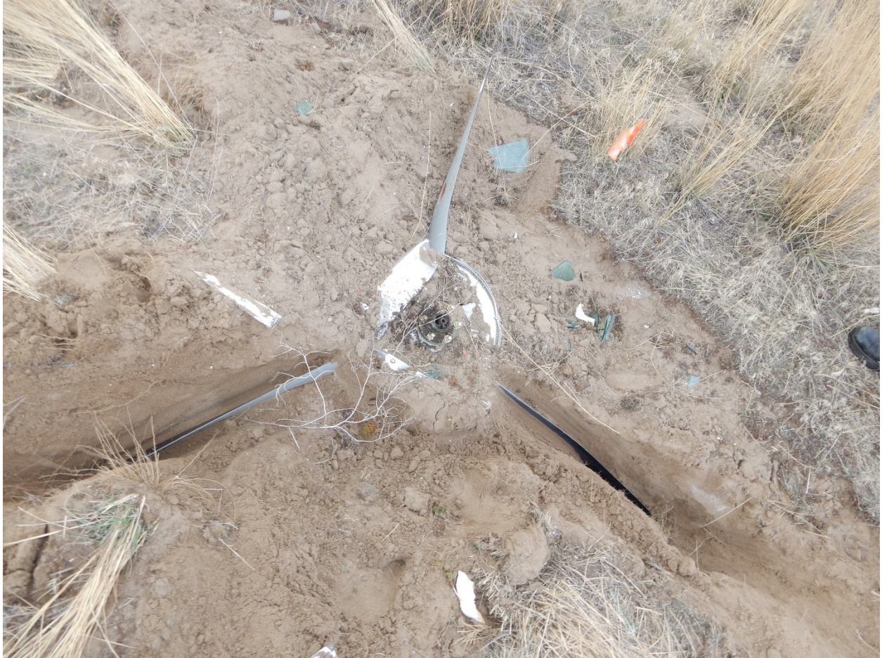
Figure 6. Propeller, as found at the accident site.
