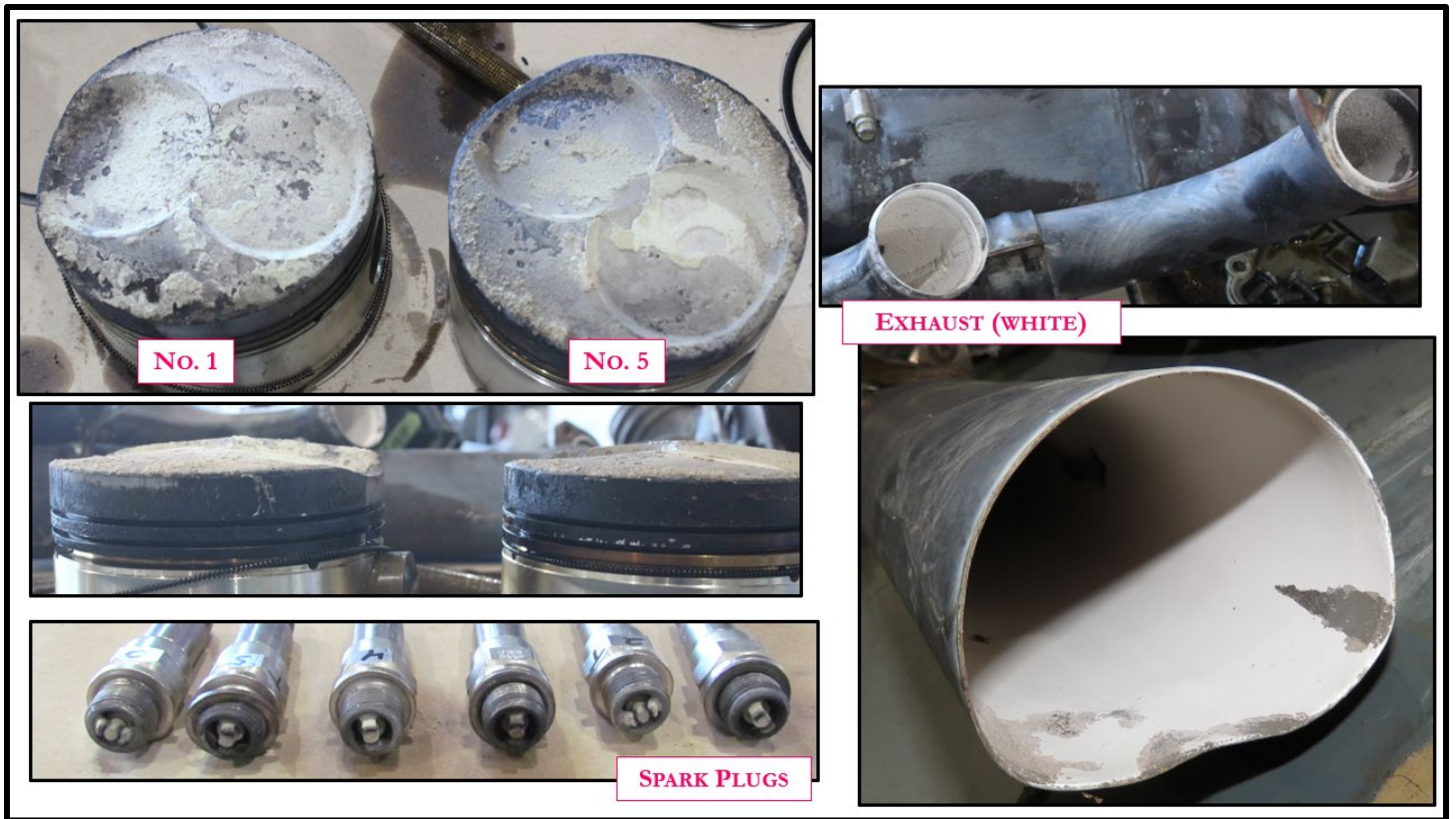
Picture 24: Combustion Signatures
