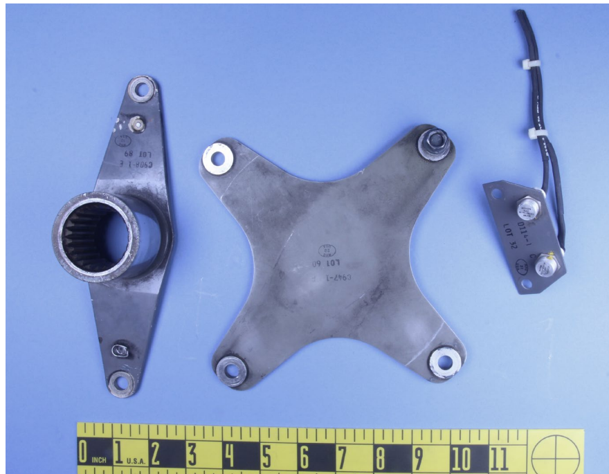
Figure 1: Tail rotor yoke with damaged magnet holder, flex plate, and hall effect sensors with holder.
