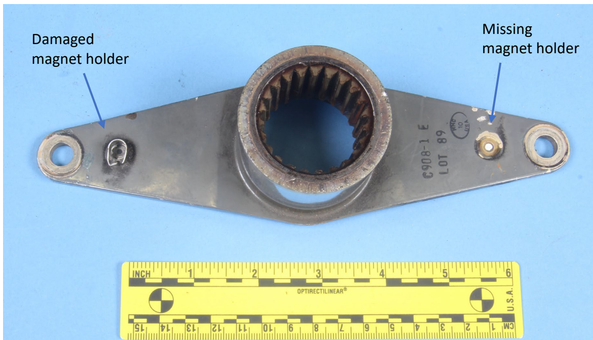
Figure 2: Tail rotor yoke with damaged magnet holder.
