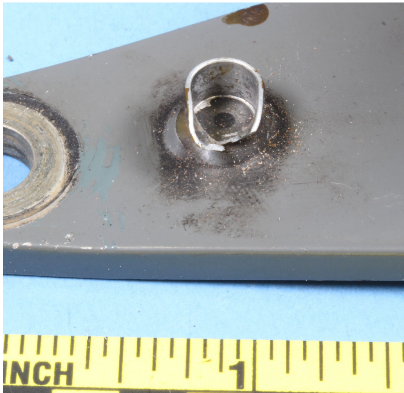
Figure 3: Fractured side of damaged magnet holder.
