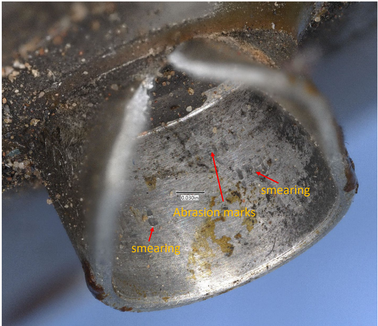
Figure 6: Interior surface of magnet holder.
