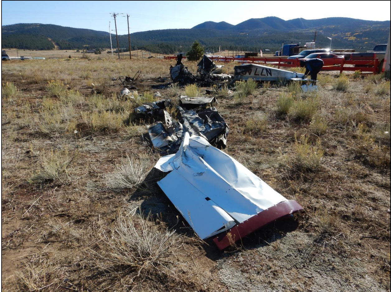
Figure 4-Accident site, main wreckage and right wing.
