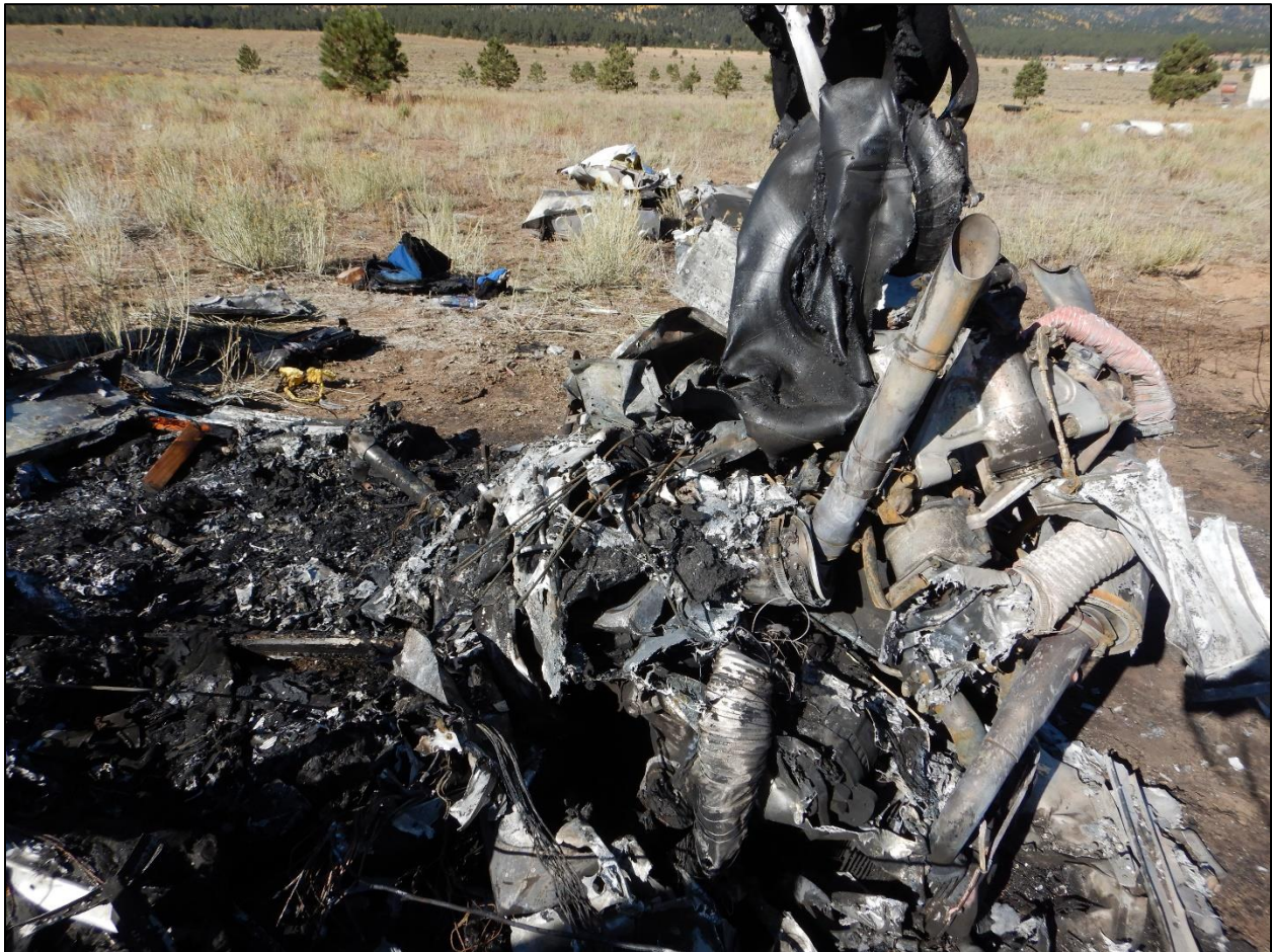
Figure 6-Accident site, forward fuselage and engine assembly.
