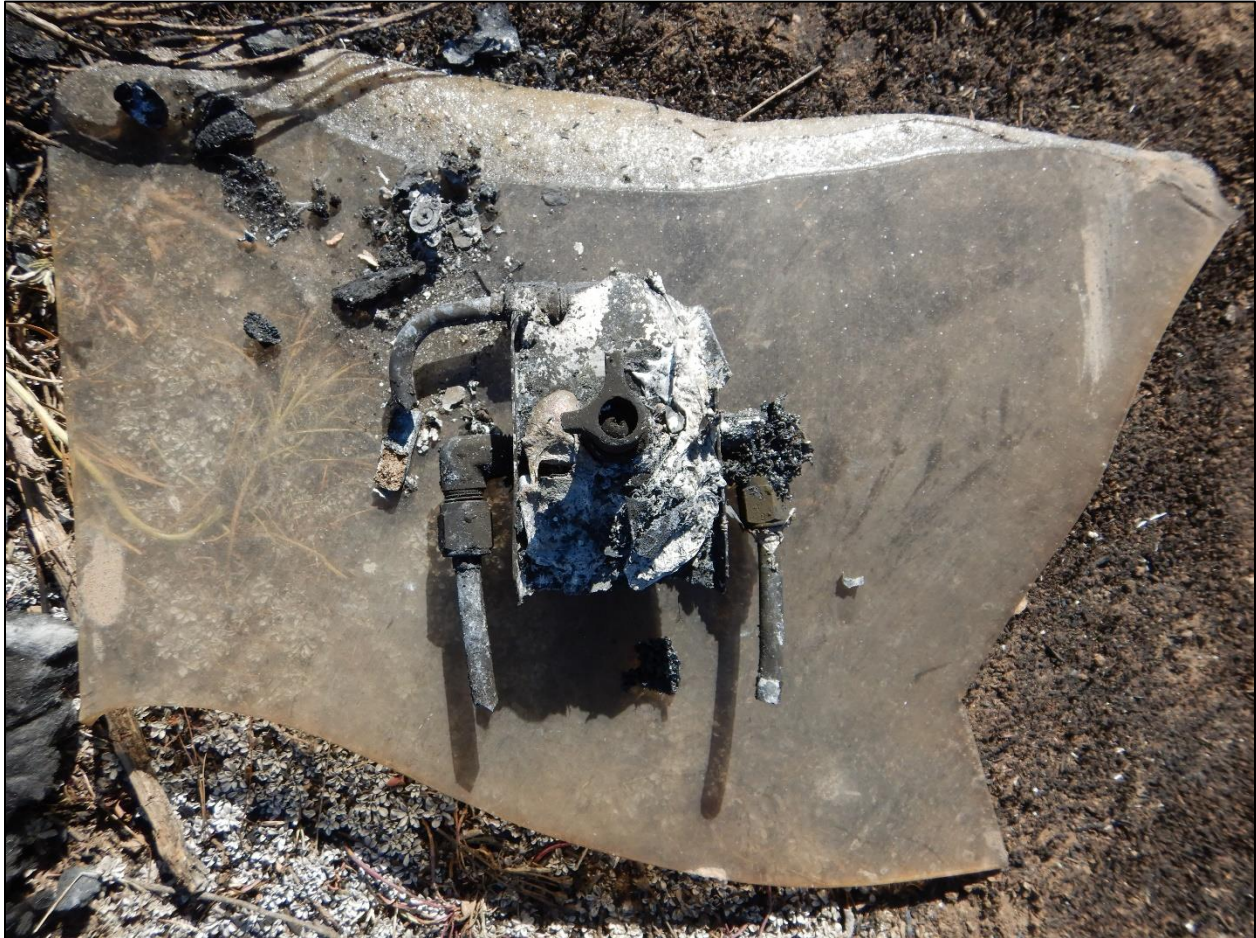
Figure 5-Accident site, fuel selector valve.
