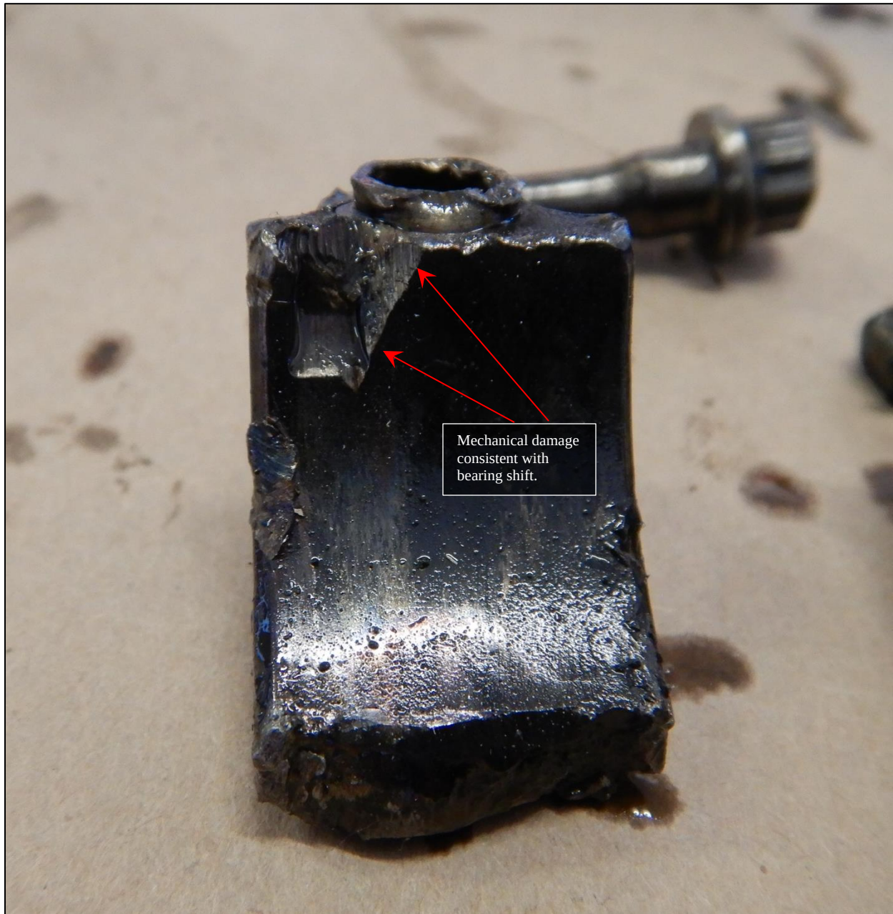
Figure 9-No. 4 connecting rod end cap section and bearing tang insert.
