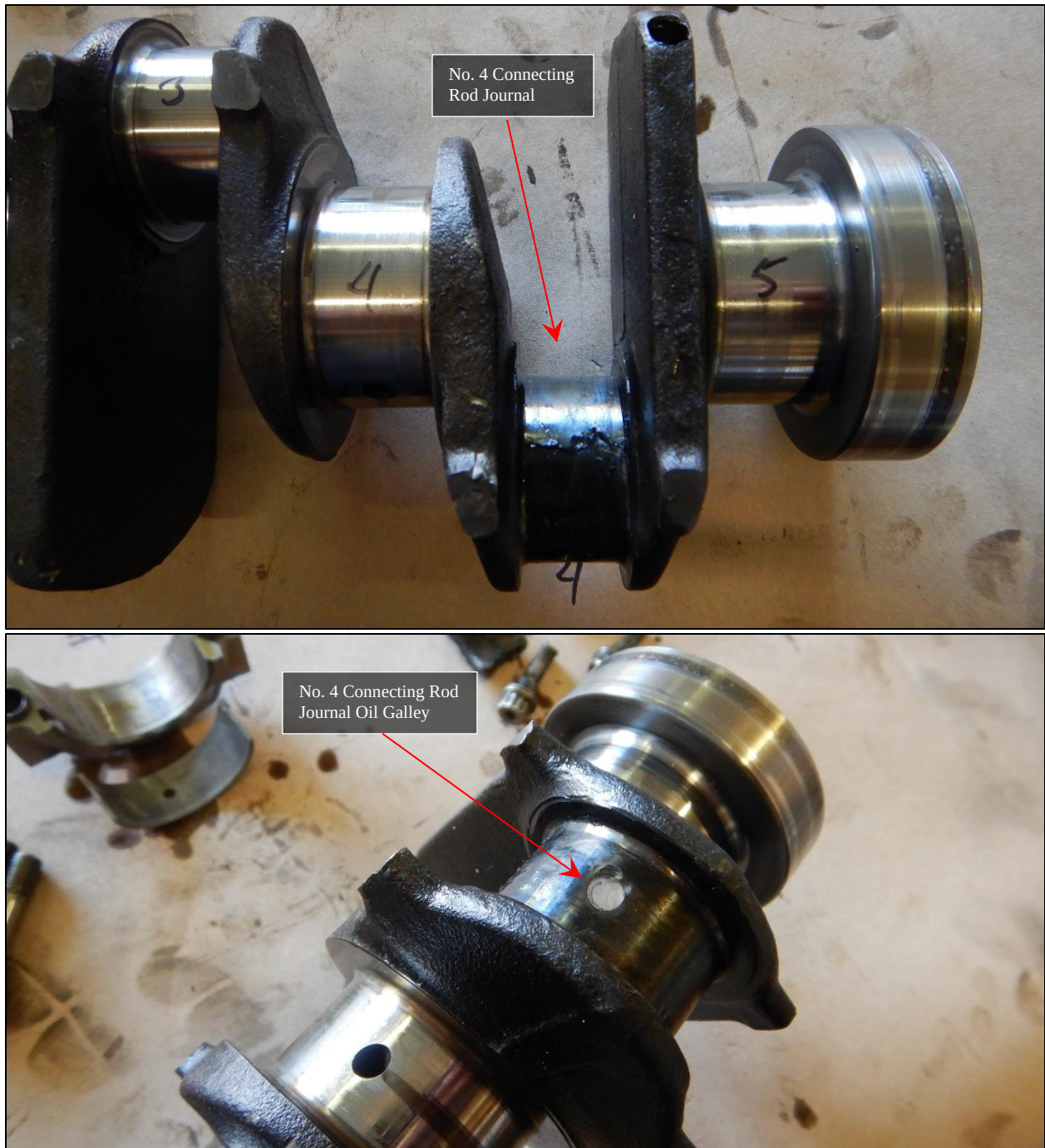
Figure 8-Crankshaft no. 4 connecting rod journal.
