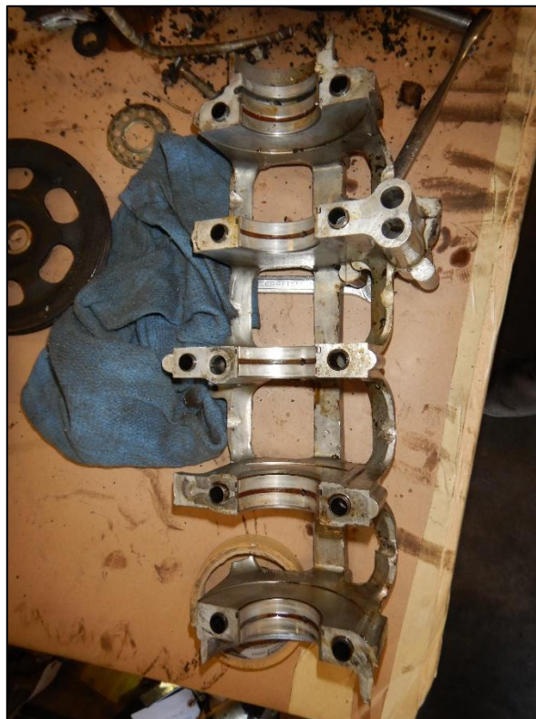
Figure 7-Lower crankshaft support and bearings.
