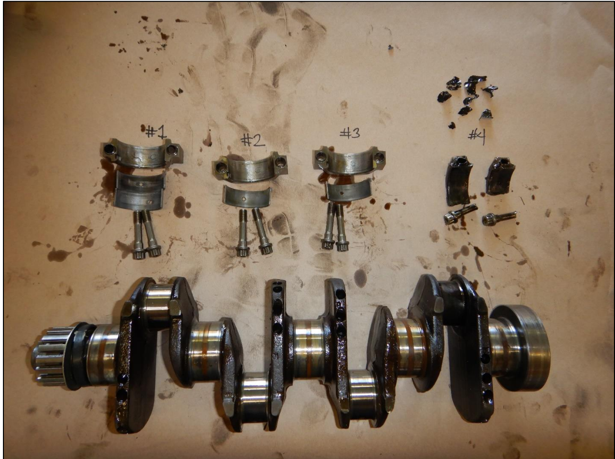
Figure 5-Crankshaft, connecting rod end caps, connecting rod bearings and bolts.
