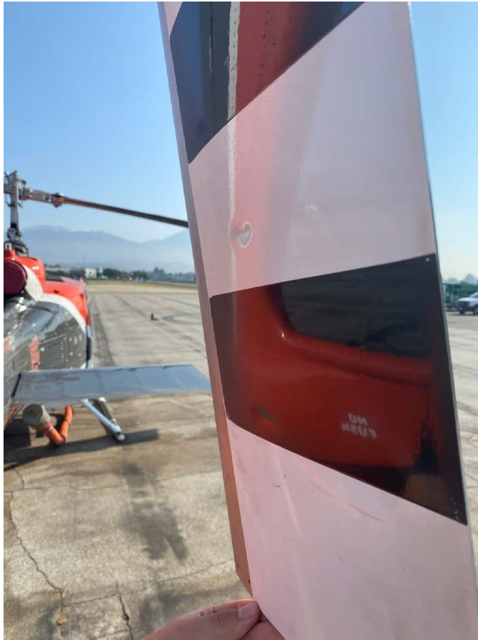
Photo 1 – View of tail rotor damage (photo courtesy of Owner)
