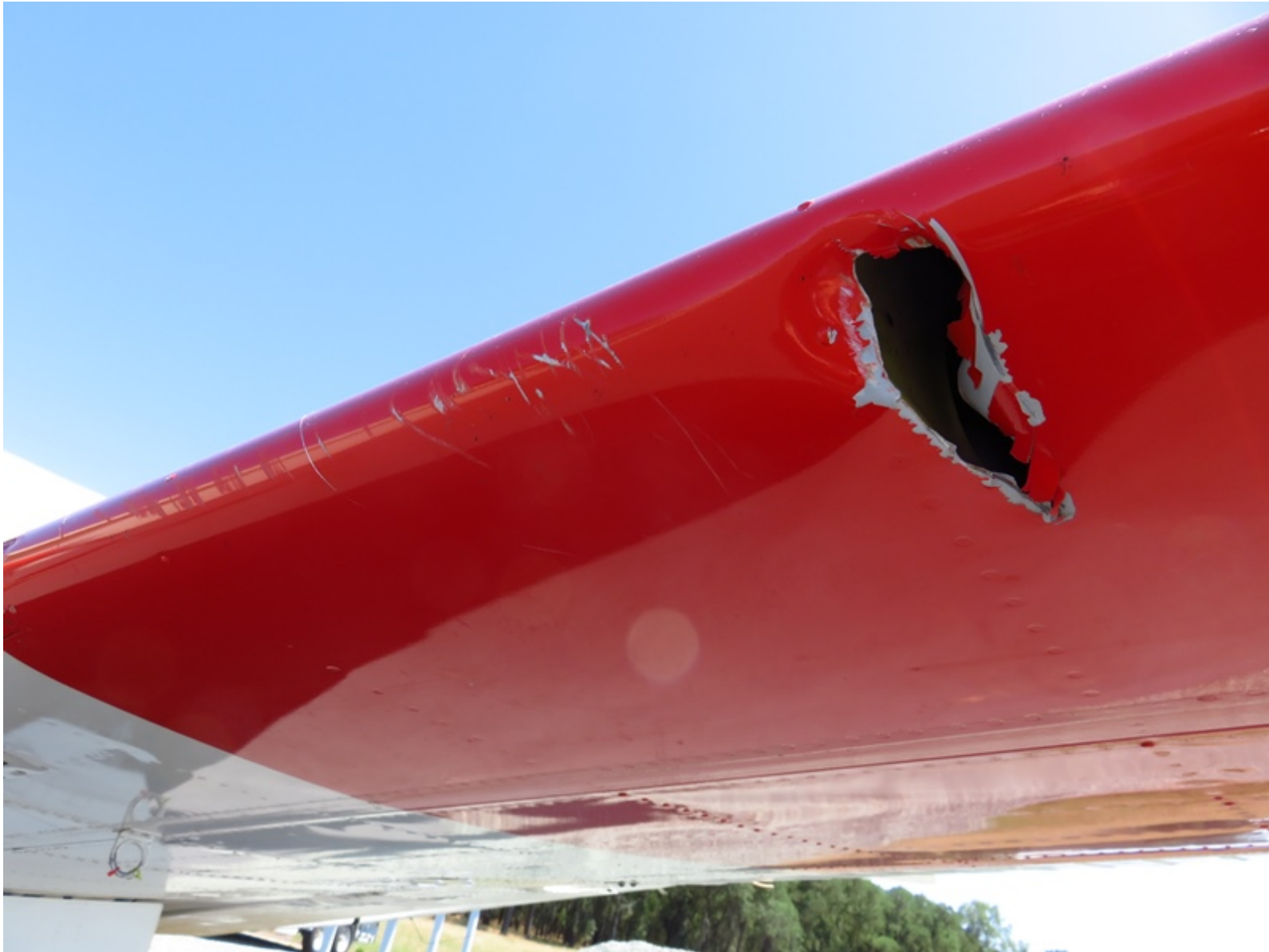
Photo 2 – Puncture and Leading Edge Damage to Left Wing
