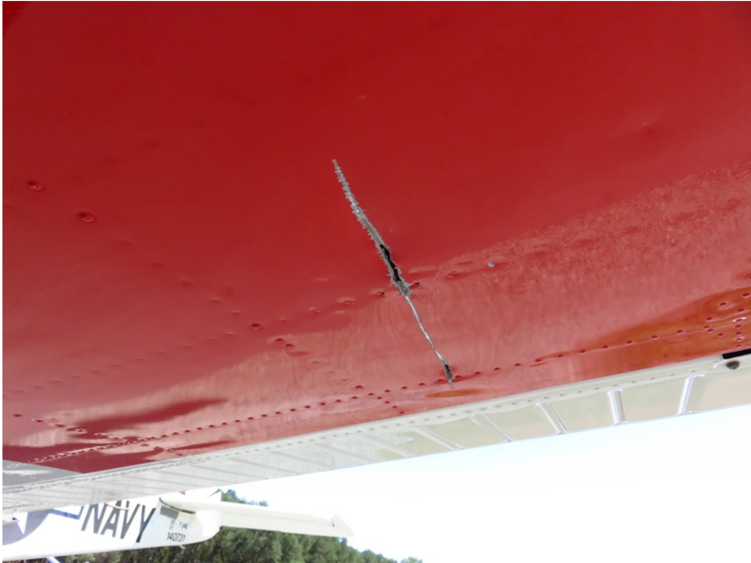
Photo 3 – Left Wing Lower Skin Damage
