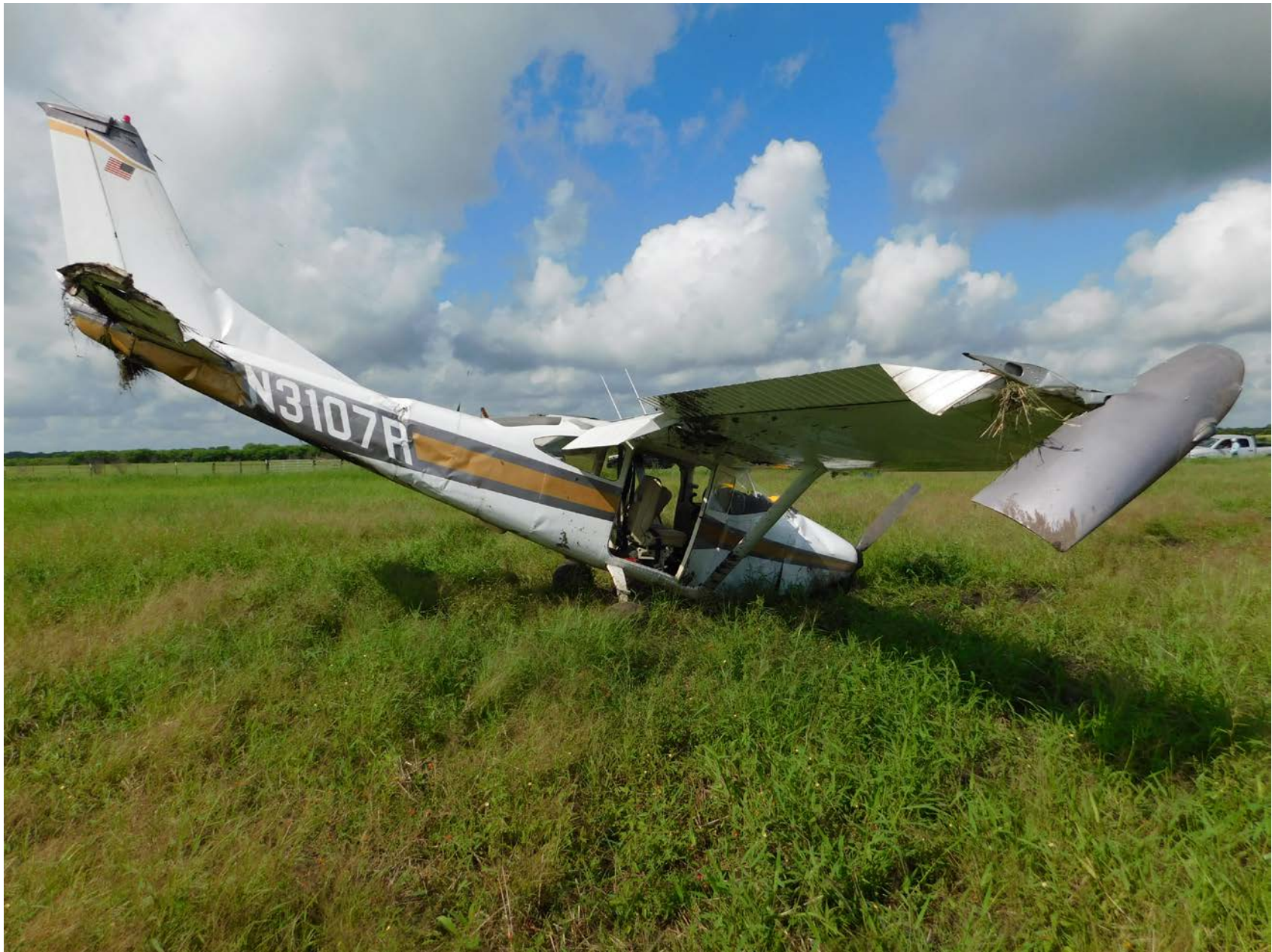
Photo 1 – View of airplane damage to fuselage (courtesy of the FAA)
