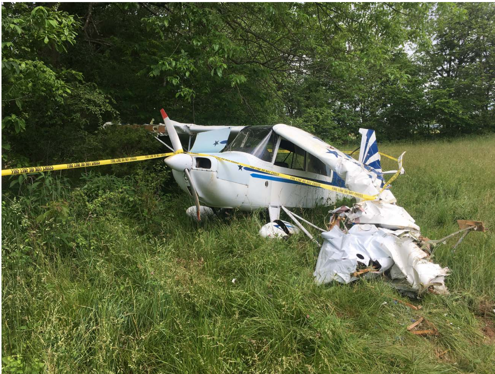
Photo 1 – View of airplane damage to both wings (courtesy of the FAA)
