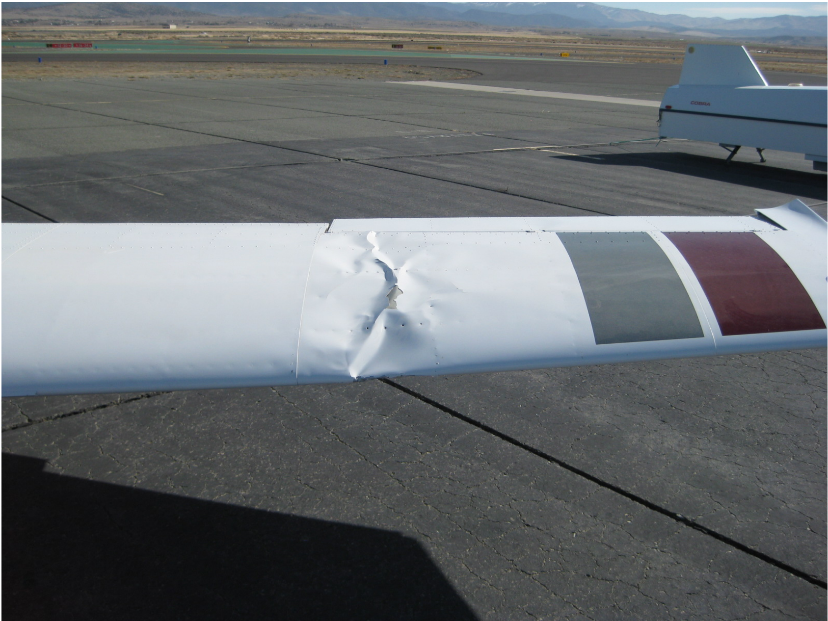
Photo 3 - Photo of the damage to the left wing. Courtesy of Airport Operations.
