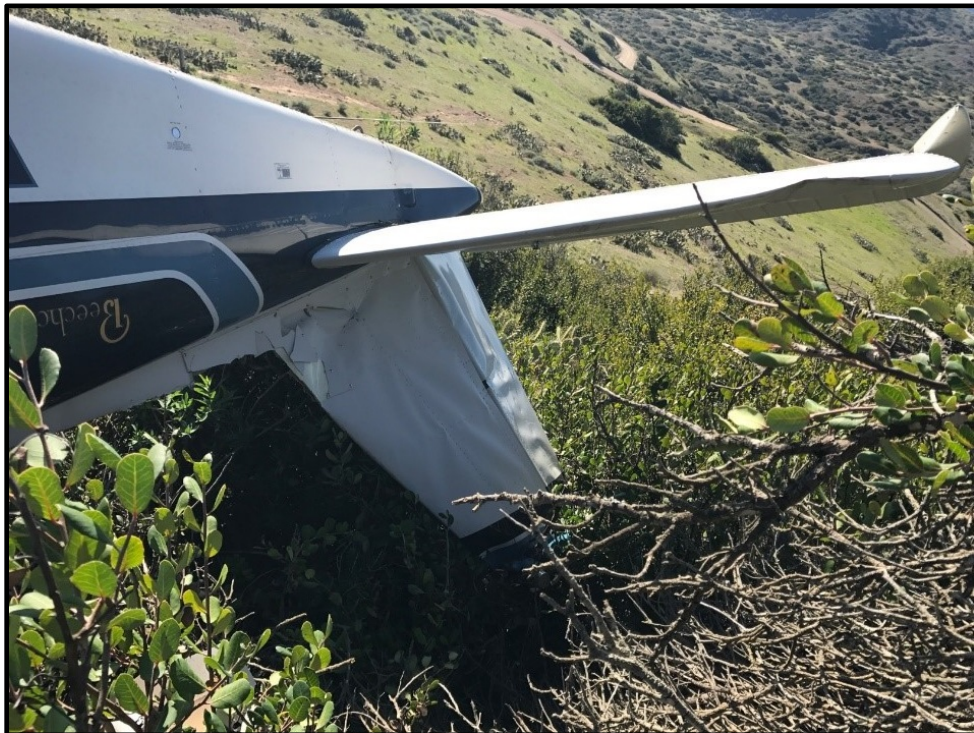
Figure 2: Airplane's damaged tail section (right side).
