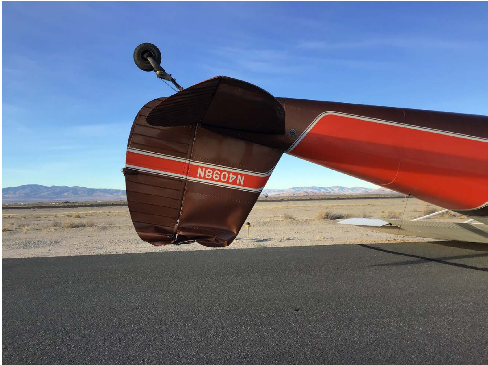
Photo 2 – Damaged vertical stabilizer
