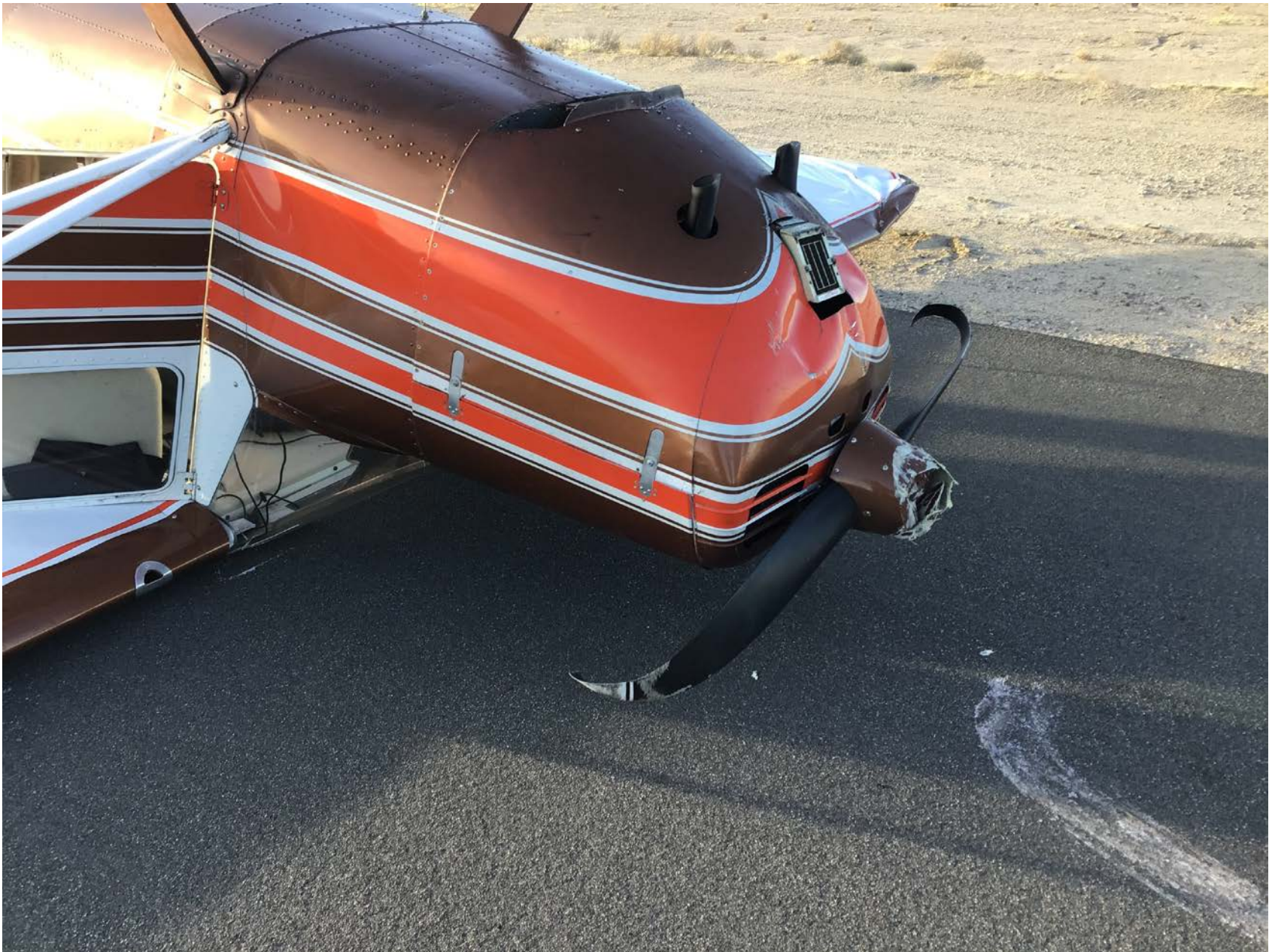
Photo 3 – Damaged propeller and right wing tip
