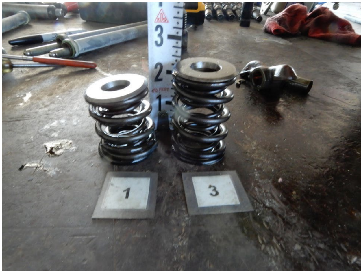
Figure 5. Number one intake valve springs compared to number three intake valve spring.
