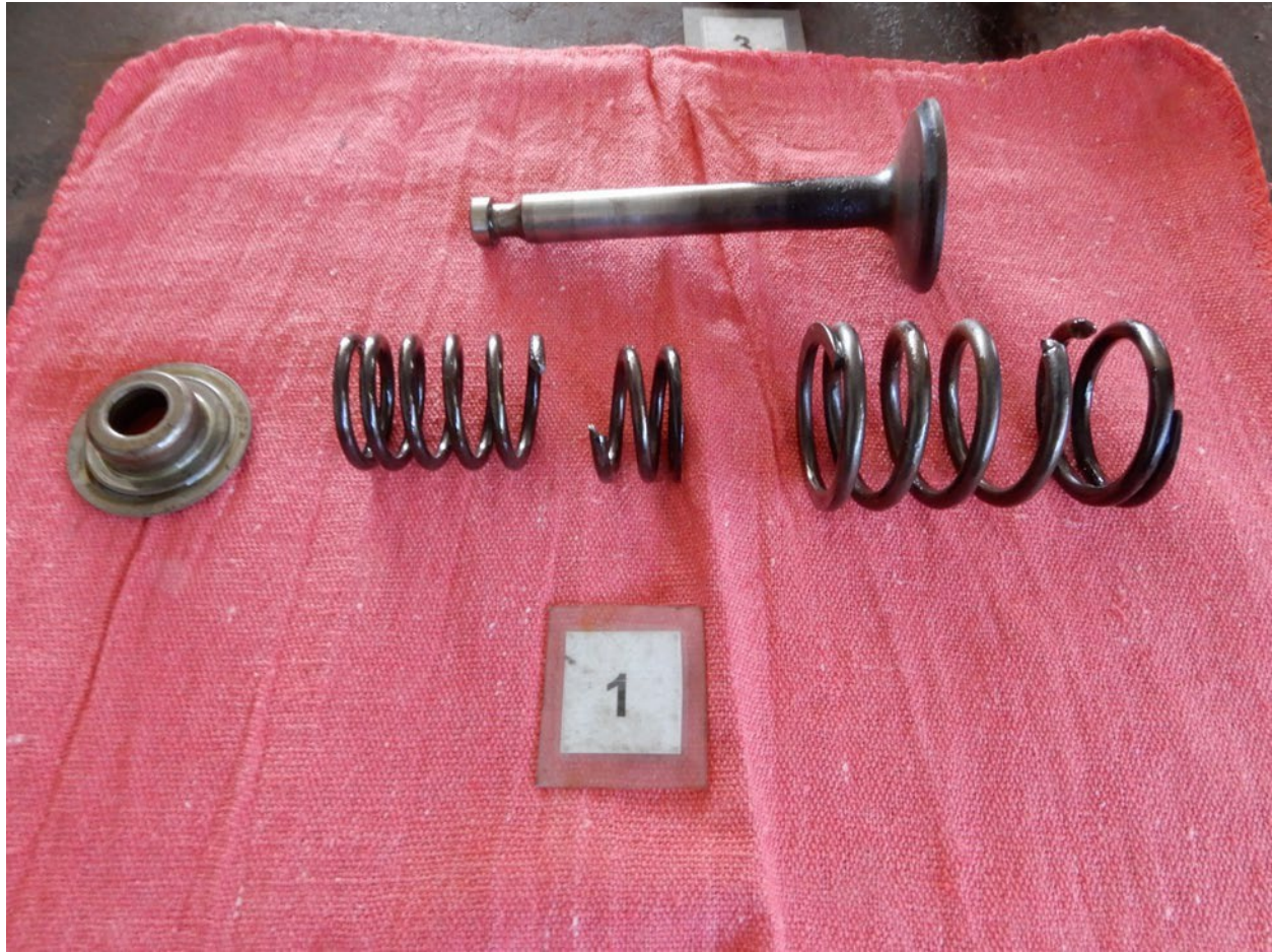
Figure 6. Number one intake valve springs showing fractures on both springs.
