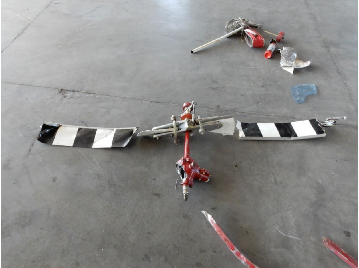
Figure 3. Tail rotor assembly and 90° gearbox.
