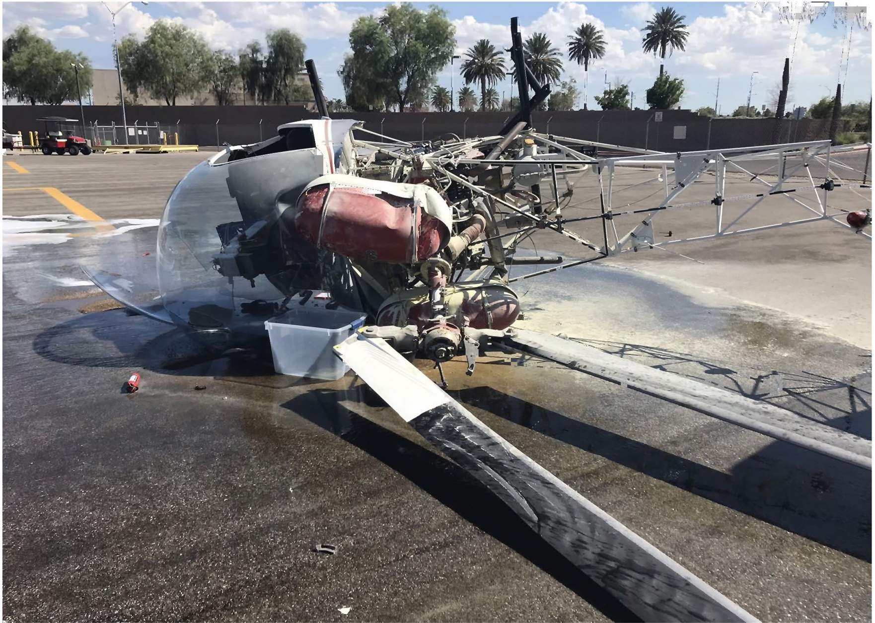
Photo 1 – N6064H, top-side view, showing damage to the fuselage, and main rotor system. Photo courtesy of the owner.
