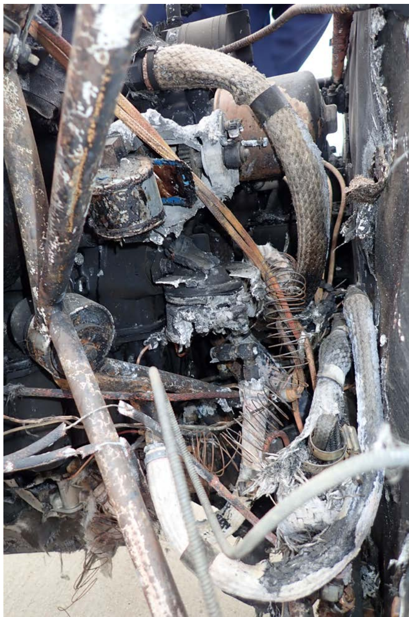
Photo 4 – Fuel Pump and Lower Left Engine Compartment
