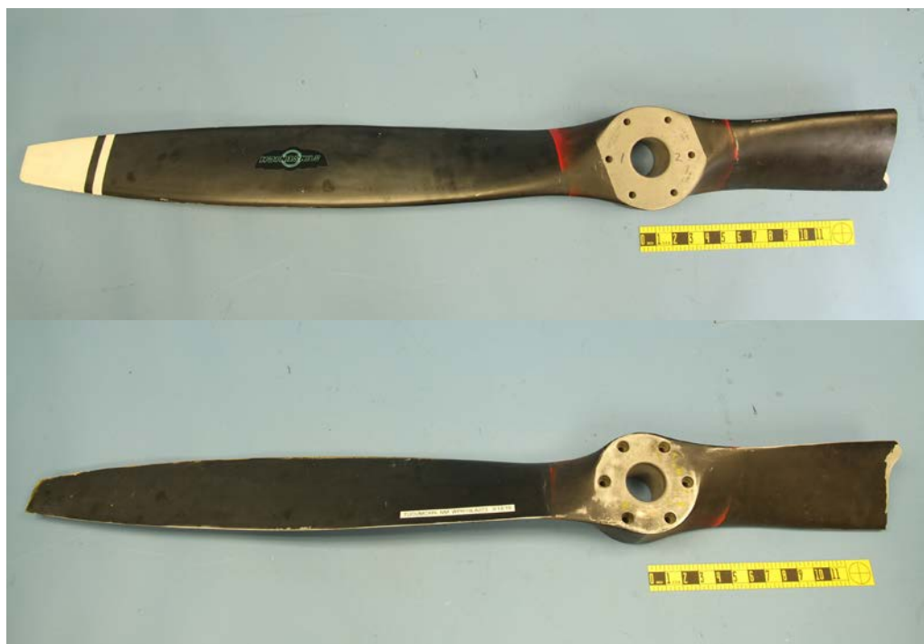
Figure 1: Portion of Sensenich propeller as received.
