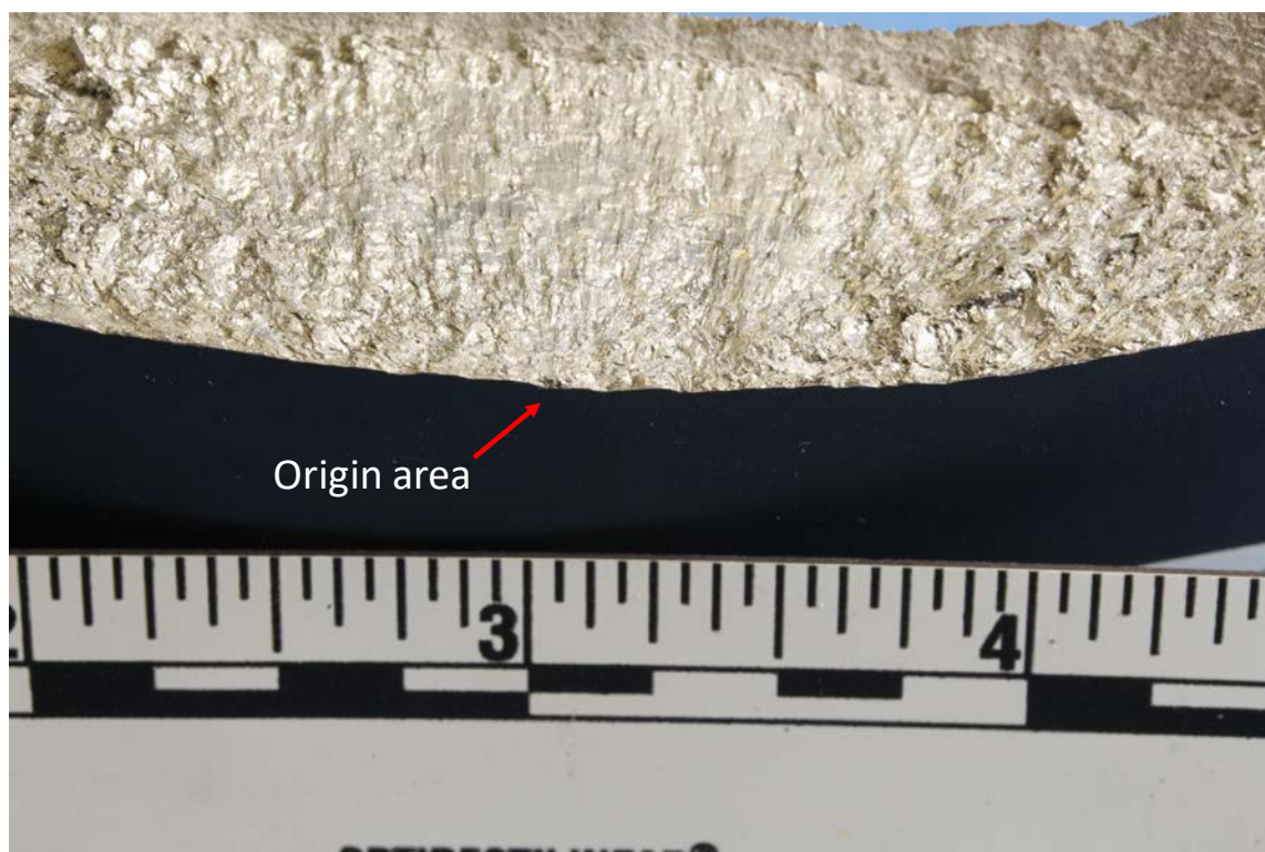
Figure 3: Origin area at the center of curvature of the flat fracture containing a small pit on the face of the propeller blade.
