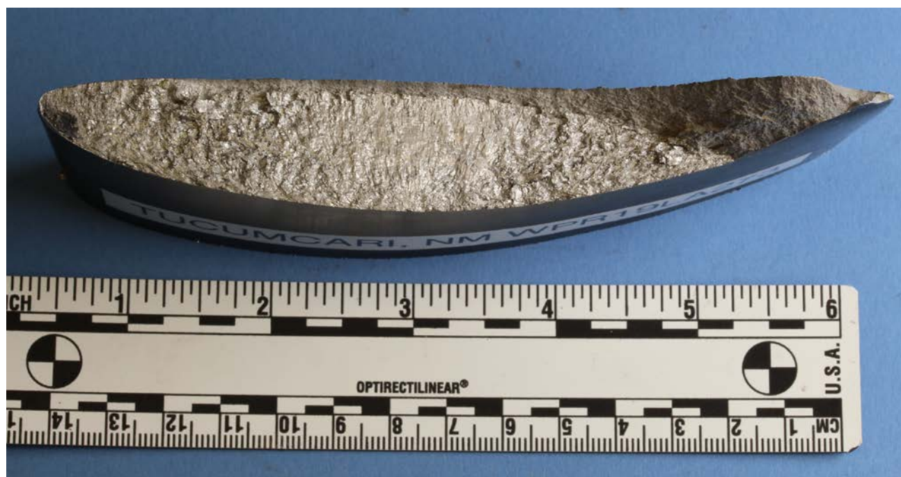
Figure 2: Section of the propeller containing the fracture surface.
