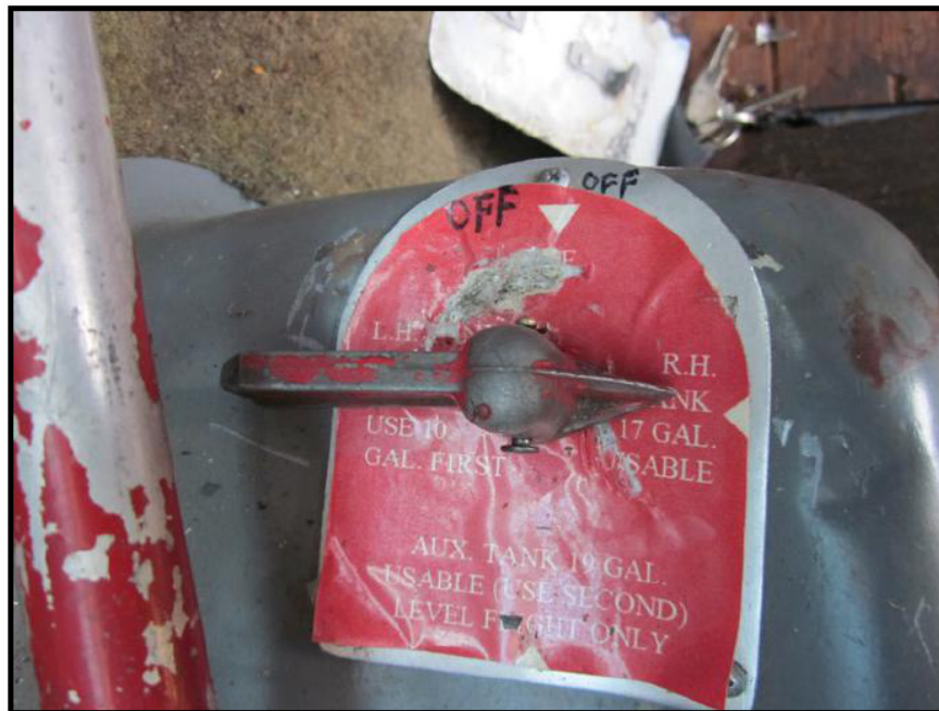
Figure 1: Fuel selector positioned to the right tank. (Courtesy of FAA)
