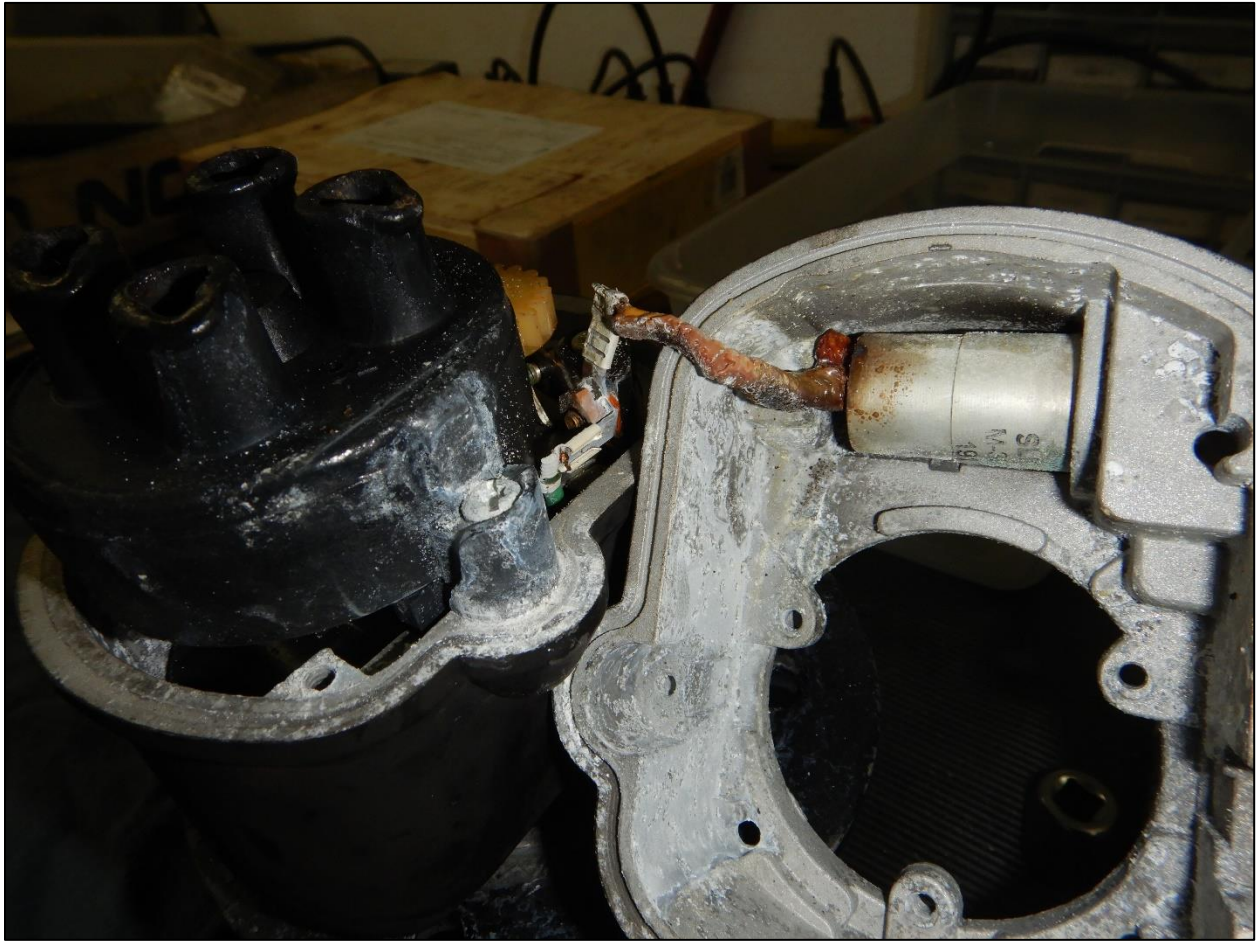
Figure 5-Left Magneto Teardown, Internal Thermal Damage
