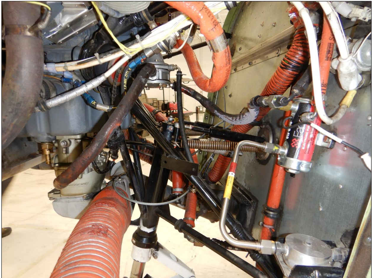
Figure 4-Accident Airplane Fuel Lines (3) Installed on an Exemplar Airplane
