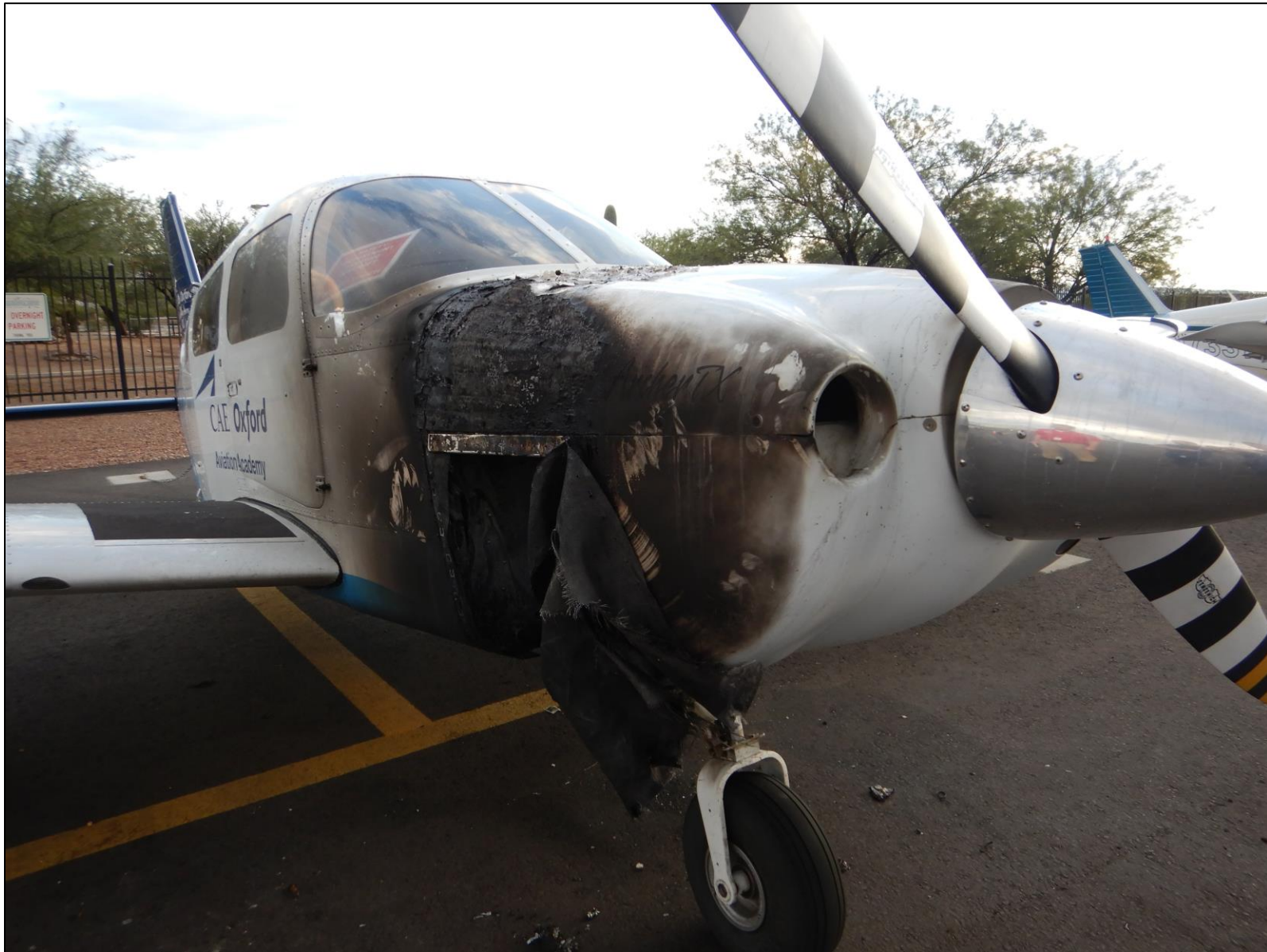
Photo 2 – Accident site, forward right side of engine cowling.
