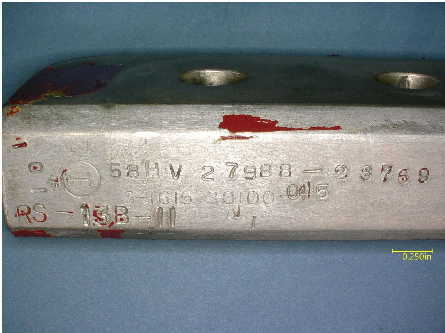
Photo 4 – Tail rotor shank showing the part number S-1516-30100-45, and the serial number, 58HV27988-28769. Photo NTSB.
