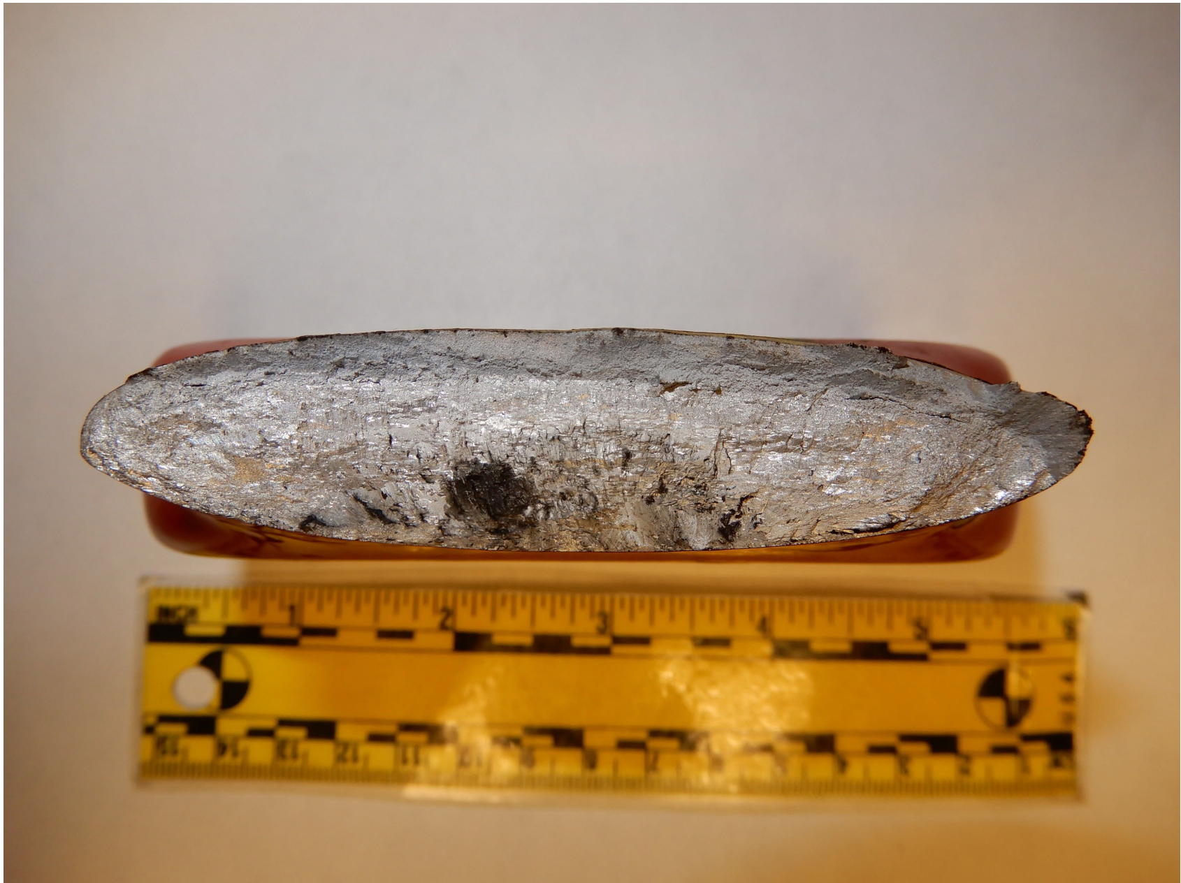
Photo 5 – View showing the fractured end of the tail rotor blade. Photo NTSB.
