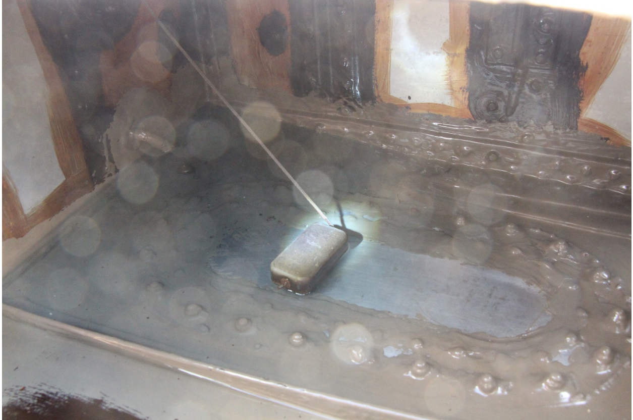
Photograph 3: Left Fuel Tank Sending Unit at Low Point In Fuel Tank
