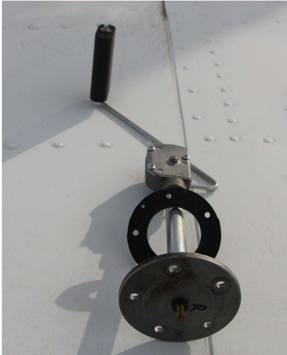
Photograph 6: Right Fuel Tank Sender
