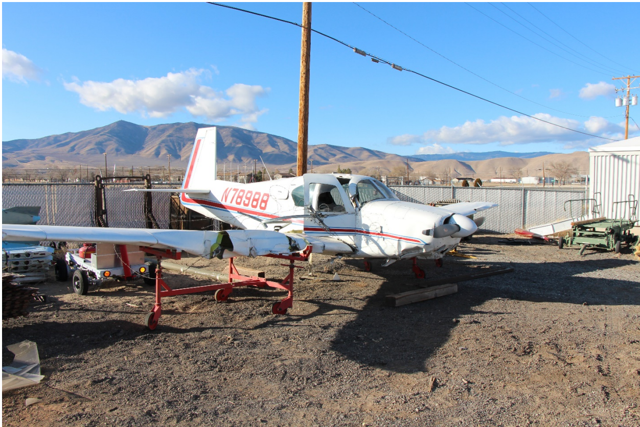
Photograph 1: Right Quartering View of Accident Airplane Showing Fence Post and Barbed Wire at Door
