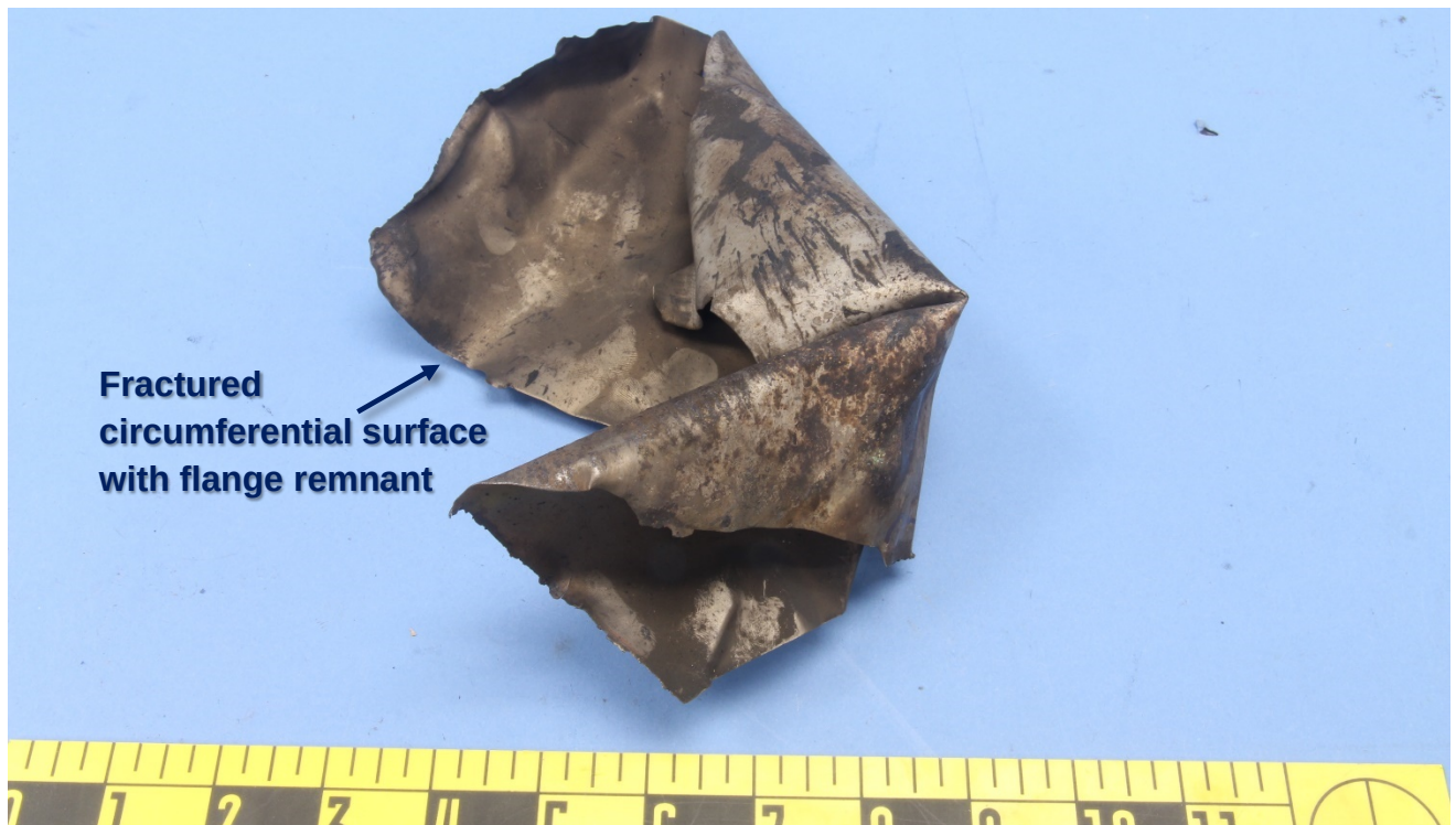
Figure 3 – View of the internal surfaces of the bleed air duct remnant.
