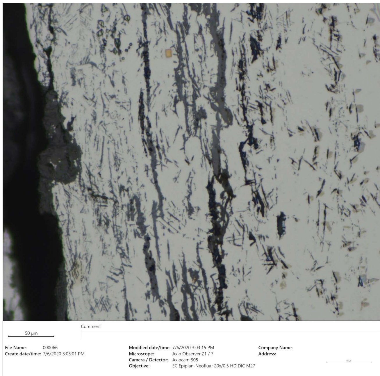
Figure 36 – BF optical micrograph of a closer look of the layered corrosion compounds in Figure 35 (~500X, as-polished).
