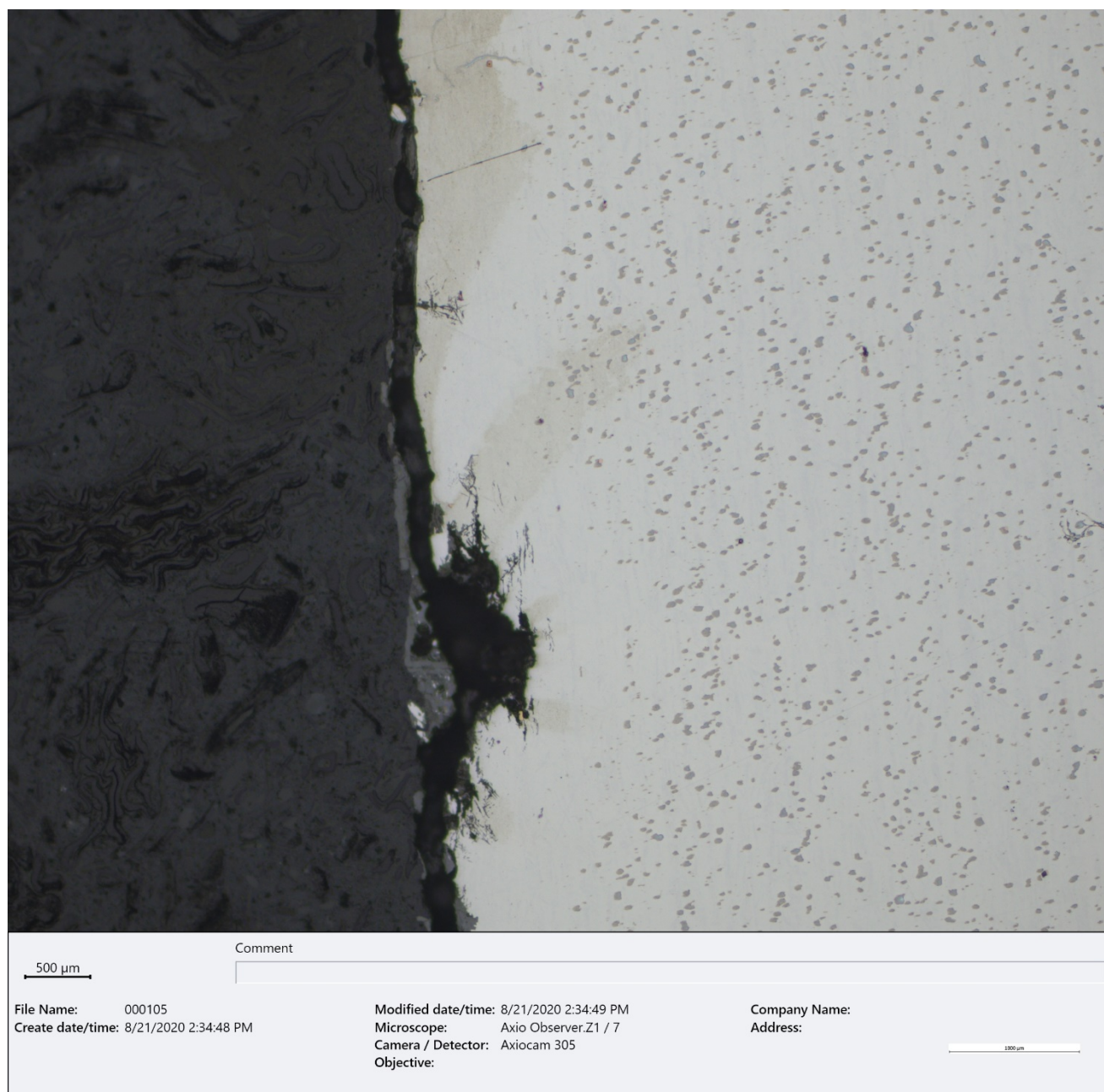
Figure 37 – BF micrograph of a surface corrosion pit on the flange piece, with branched cracking (~200X, as-polished).
