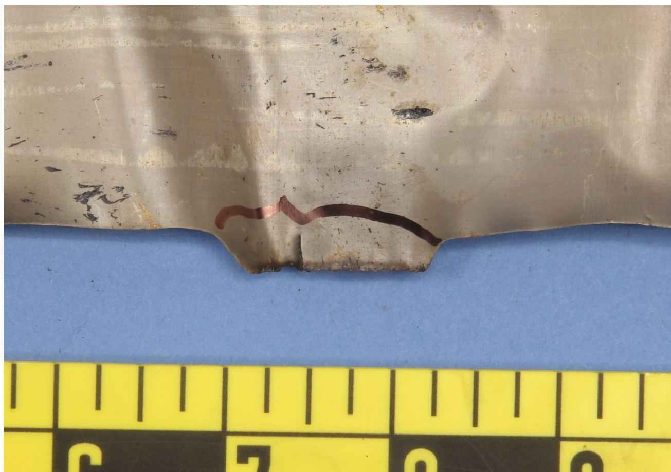
Figure 10 – The largest area of a downward-protruding portion of the bottom fracture surface of the duct remnant, which mates with the largest flat fracture area on the flange (Figure 11).
