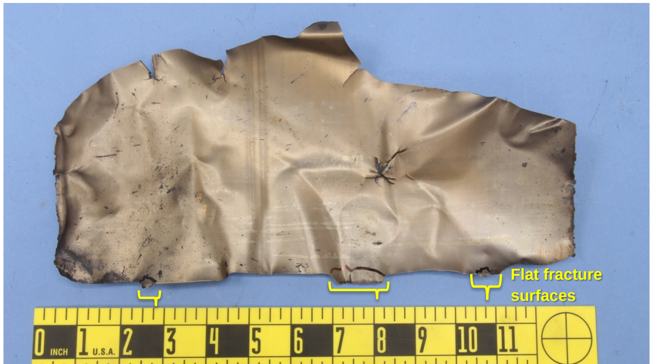
Figure 9 – View of the inside surface of the flattened duct remnant, after cleaning. The fracture surface mating the flange remnants faces downward in the figure.
