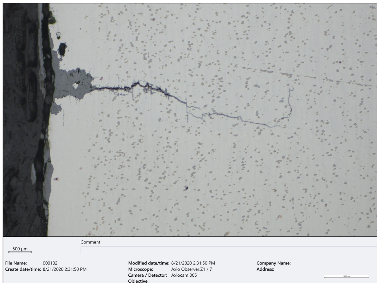
Figure 33 – BF micrograph of the horizontal crack in Figure 32, showing vertical intergranular branching (~500X, as-polished).
