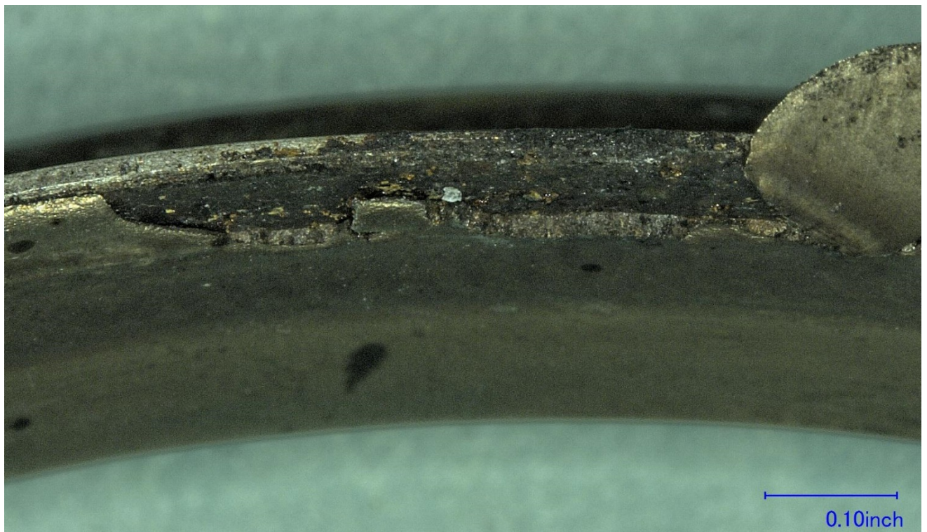
Figure 15 – Closer view of the flat fracture region shown in Figure 13.
