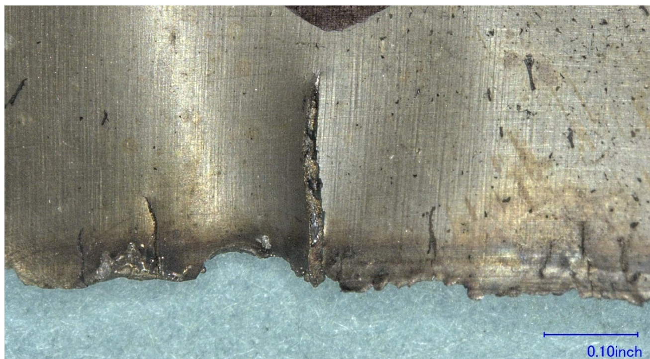
Figure 16 – Closer view of the larger flat fracture region of the duct from Figure 10.
