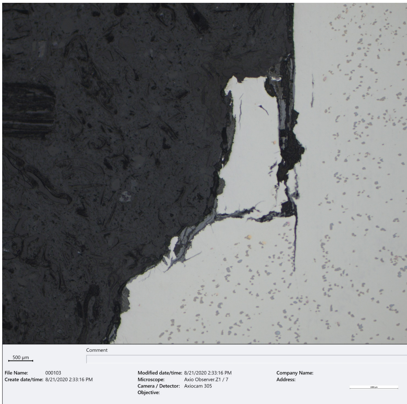
Figure 34 – BF optical micrograph showing vertical and horizontal cracking at the flat fracture surface (~200X, as-polished).
