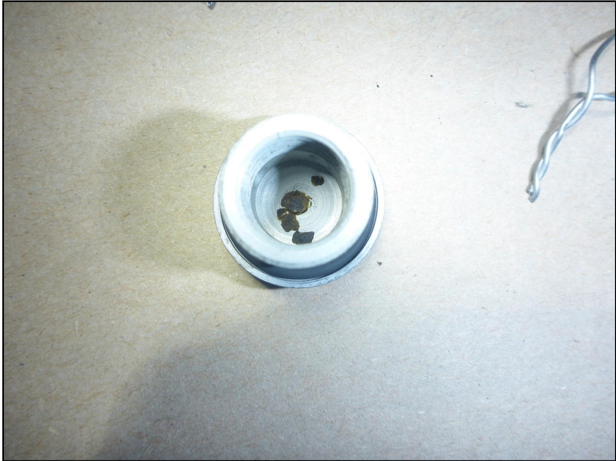
Figure 2: Contamination in carburetor float bowl for cylinder nos. 2 and 4.
