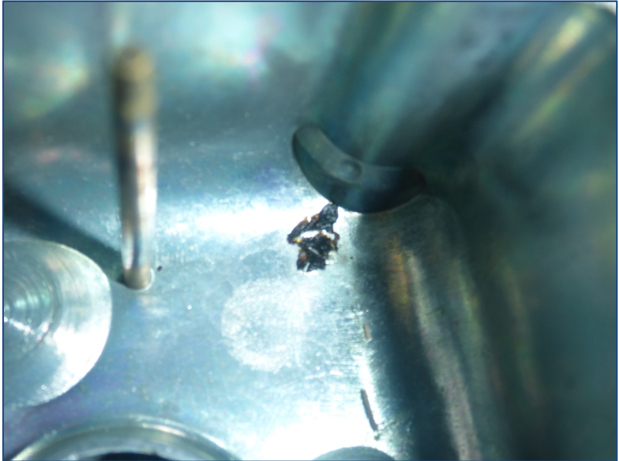
Figure 1: Contamination carburetor float bowl for cylinder nos, 1 and 3.
