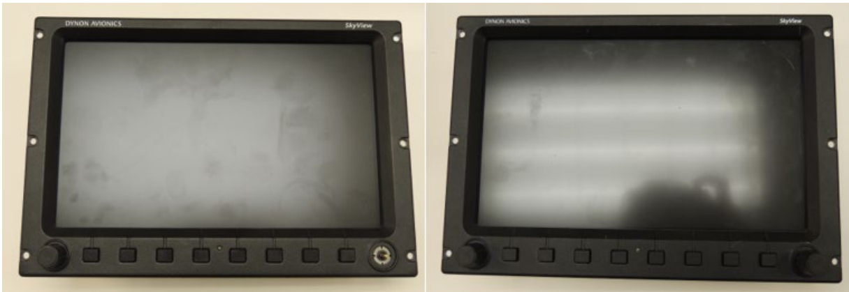
Figure 2: Dynon SV-D1000 units as received, the PFD (left) and the MFD (right).
