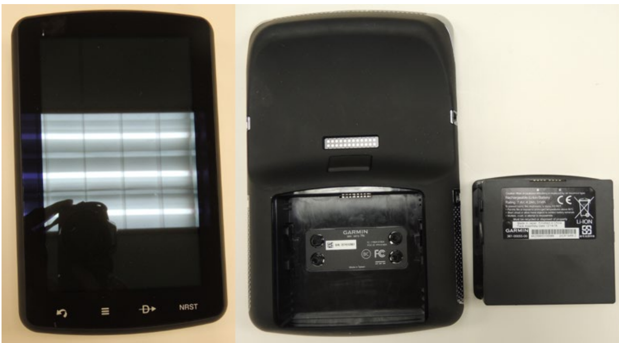
Figure 1: Front and back view of Garmin Aera 796 as received.
