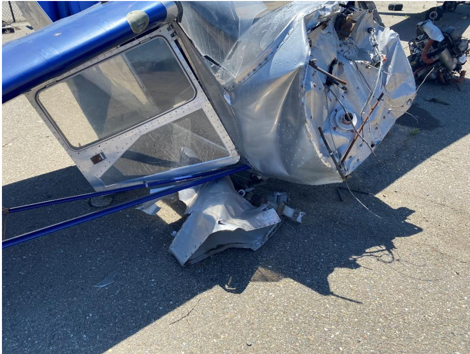
Figure 1: Damage to the Firewall and Forward Fuselage of the Airplane
