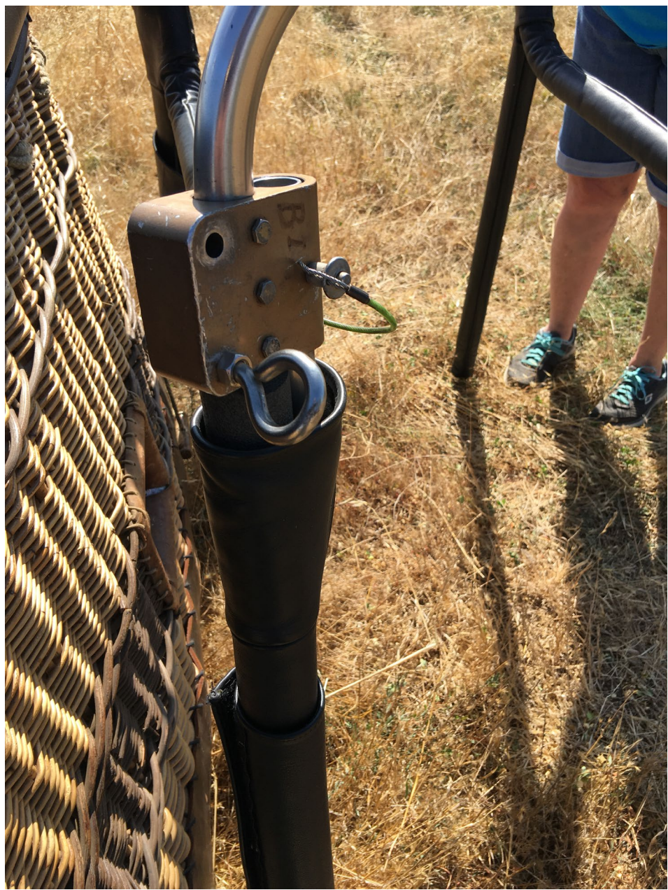
Photo 2 – Corner Plate with intact Eyelet at Accident Site (Photo Courtesy of Fire Department)
