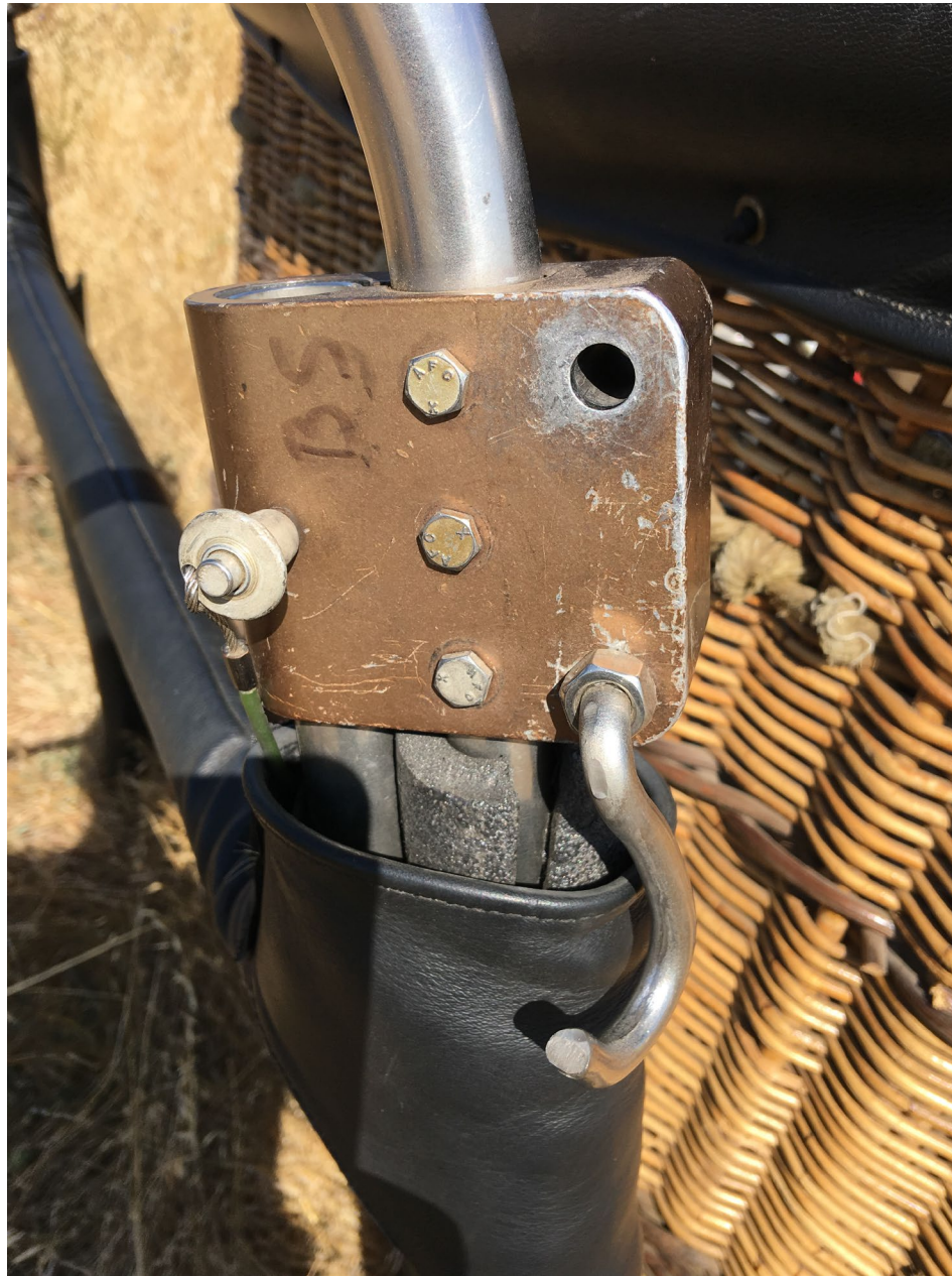
Photo 4 – Corner Plate with Elongated Eyelet Screw at Accident Site (Photo Courtesy of Fire Department)
