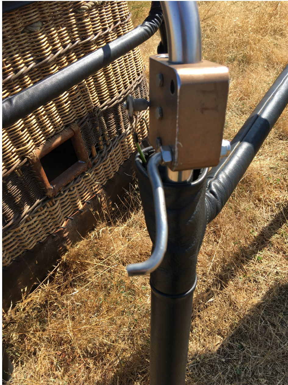
Photo 5 – Corner Plate with Elongated Eyelet Screw at Accident Site (Photo Courtesy of Fire Department)
