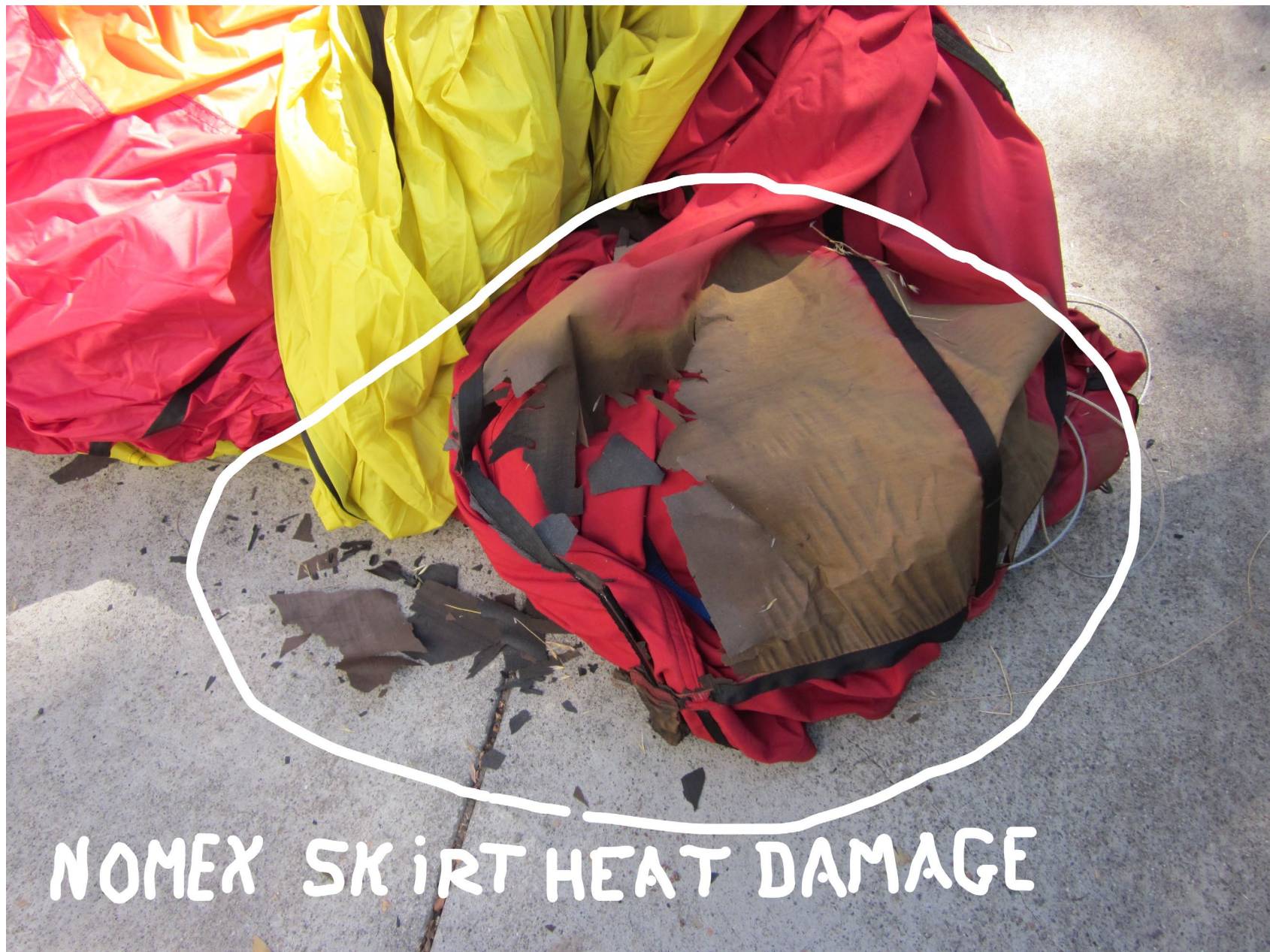
Photo 9 – Nomex Skirt Heat Damage (Photo Courtesy of FAA)
