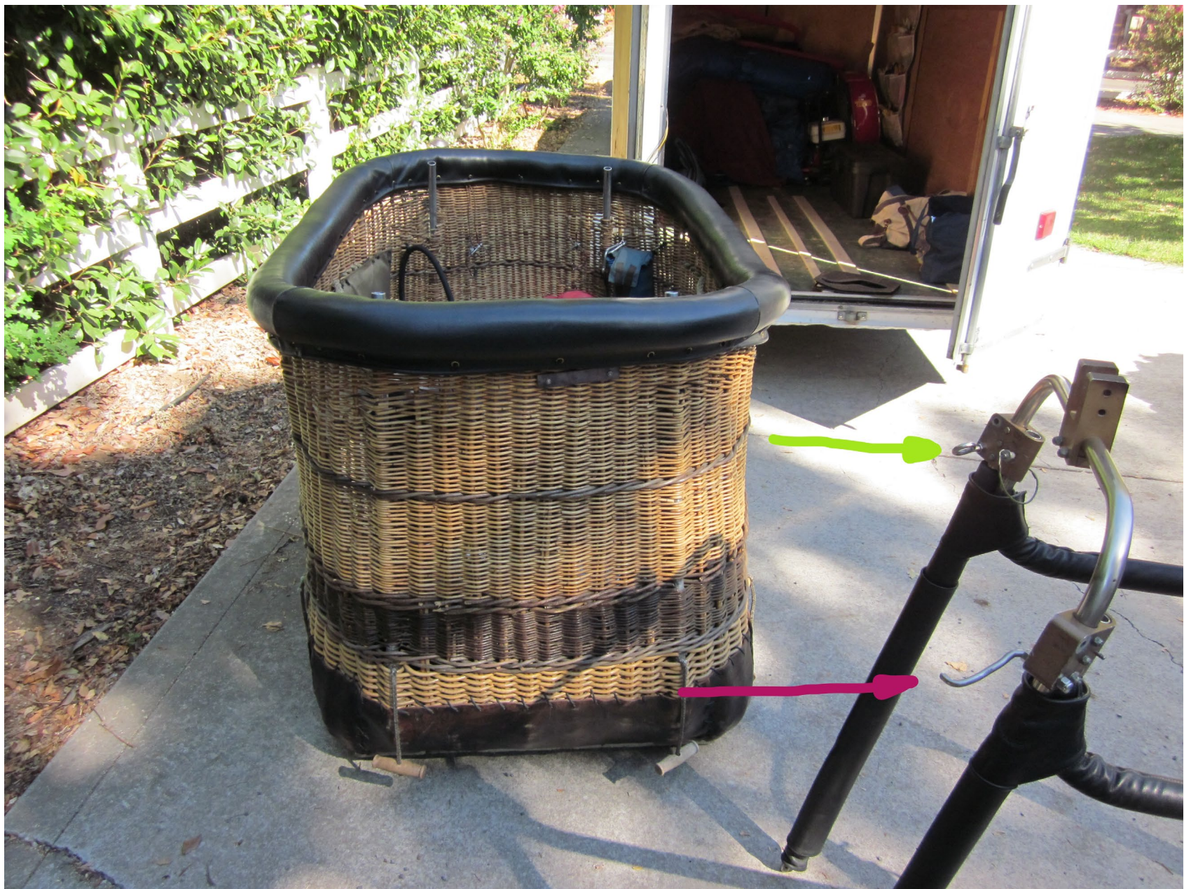
Photo 7 – View of Rigid Frame (Photo Courtesy of FAA)
