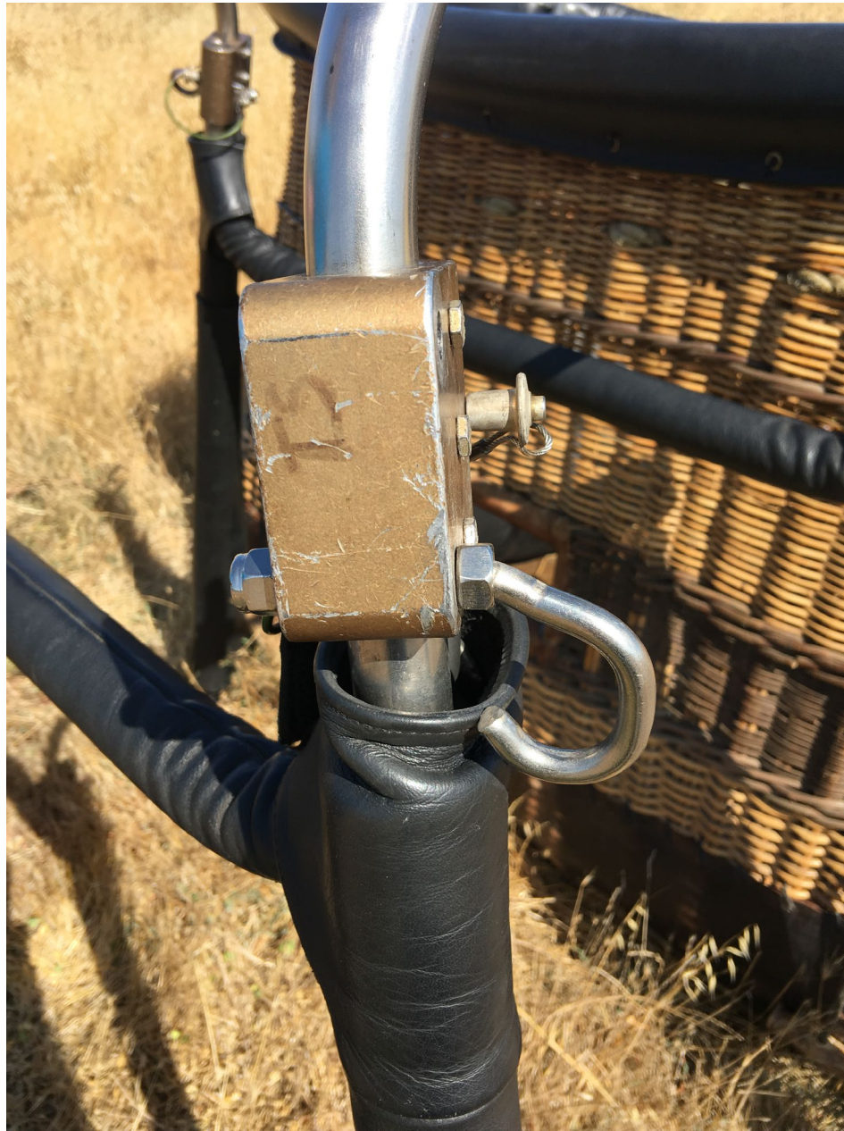
Photo 3 – Corner Plate with Elongated Eyelet at Accident Site (Photo Courtesy of Fire Department)
