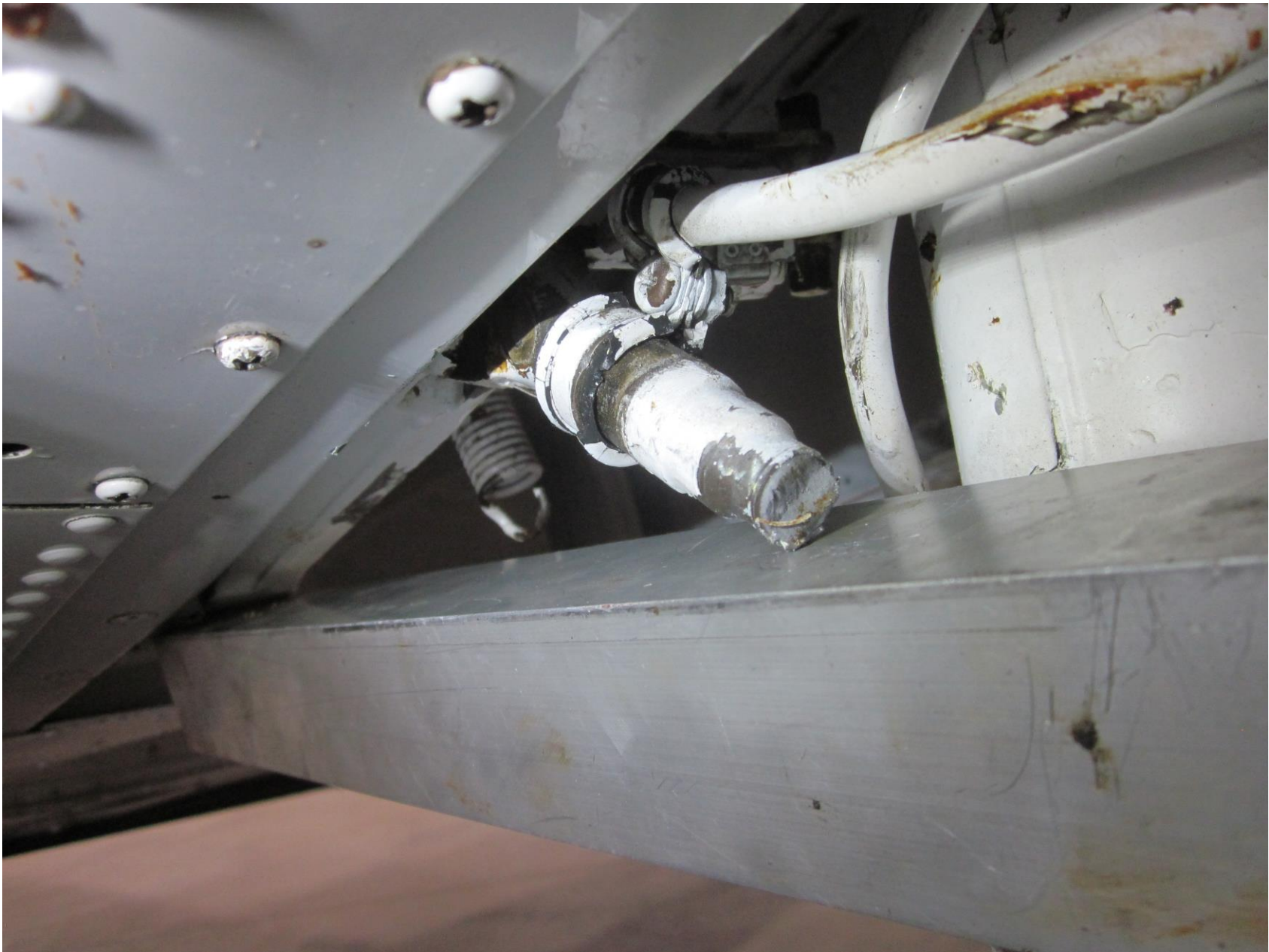
Photo 5 – Nose landing gear steering control rod. (Courtesy of the FAA)
