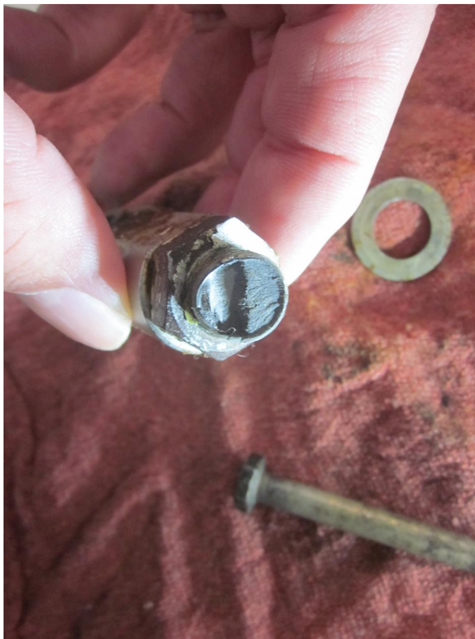
Photo 6 - Nose landing gear steering control rod, separation surface. (Courtesy of the FAA)
