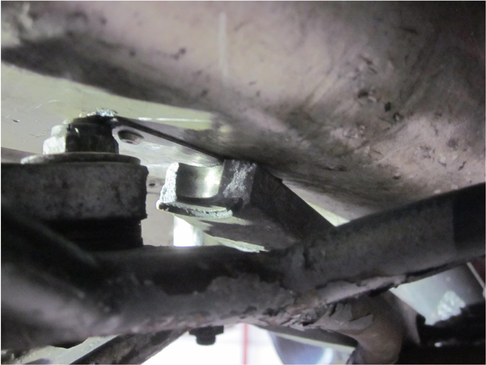
Photo 8 – Nose landing gear steering assembly, linkage separation. (Courtesy of the FAA)
