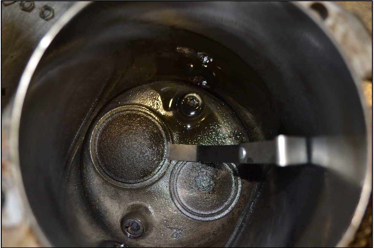
Figure 2: Interior of the No. 3 cylinder, intake valve with gap measured by the feeler gauge tool.
