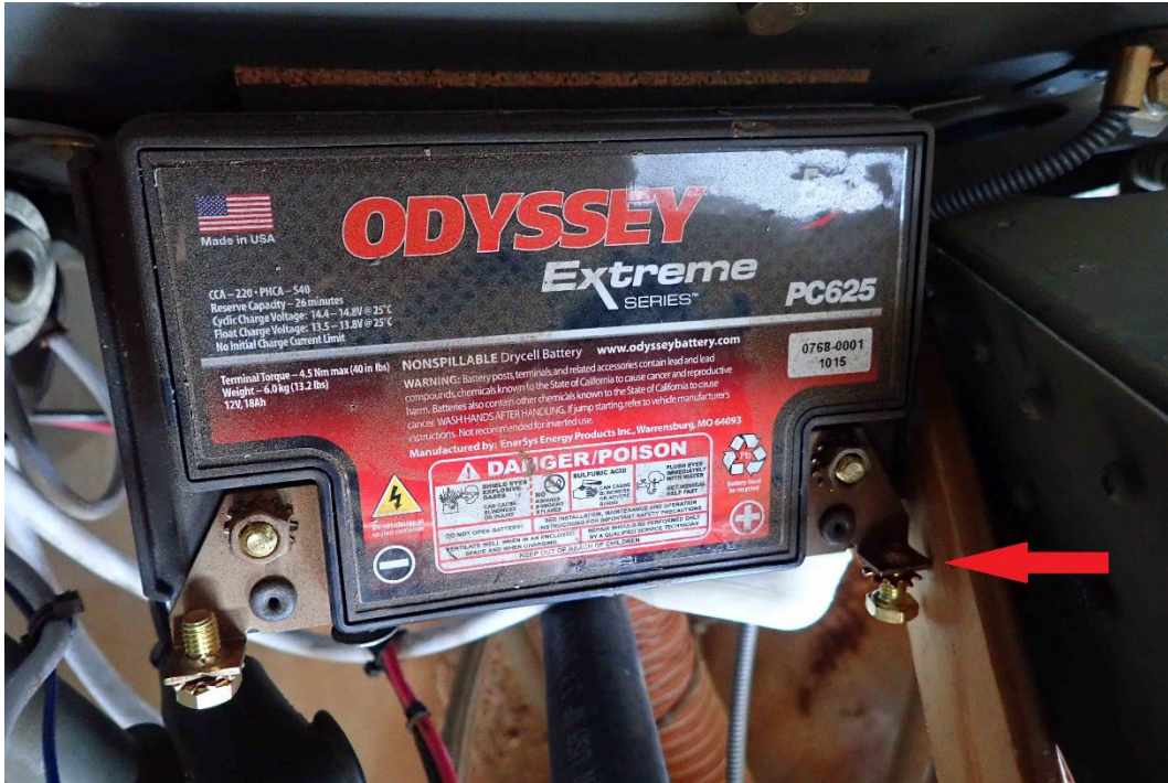
Photo 7 – Battery, red arrow indicates contact with airframe (wood block installed post-accident to prevent further damage)
