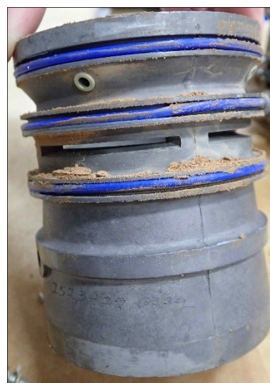
Figure 6 - Dust on Venturi Sleeve - NTSB
