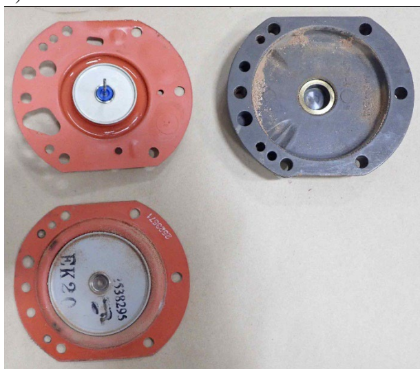
Figure 5 - Dust on Diaphragms and Housing - NTSB
