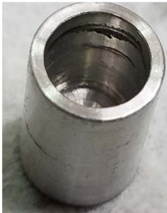
Figure XII Image of Relief Valve Poppet
