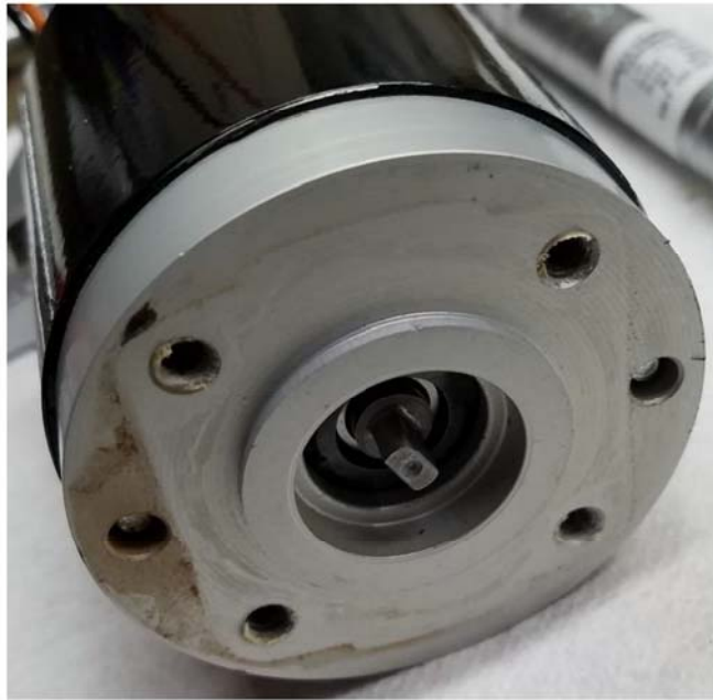
Figure XIII Image of Motor Assembly's Drive End
