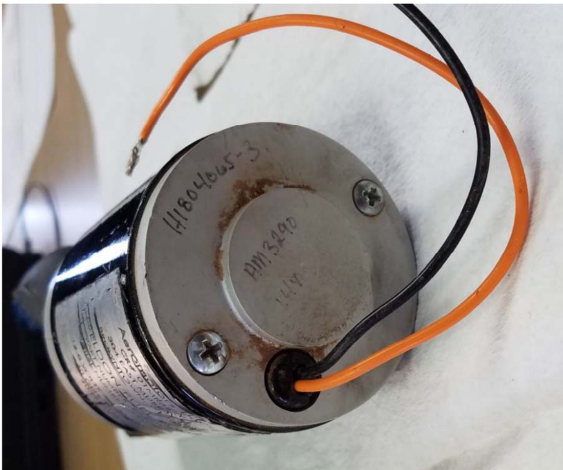
Figure VI Lead Wire End View of Pump-Motor Assembly
