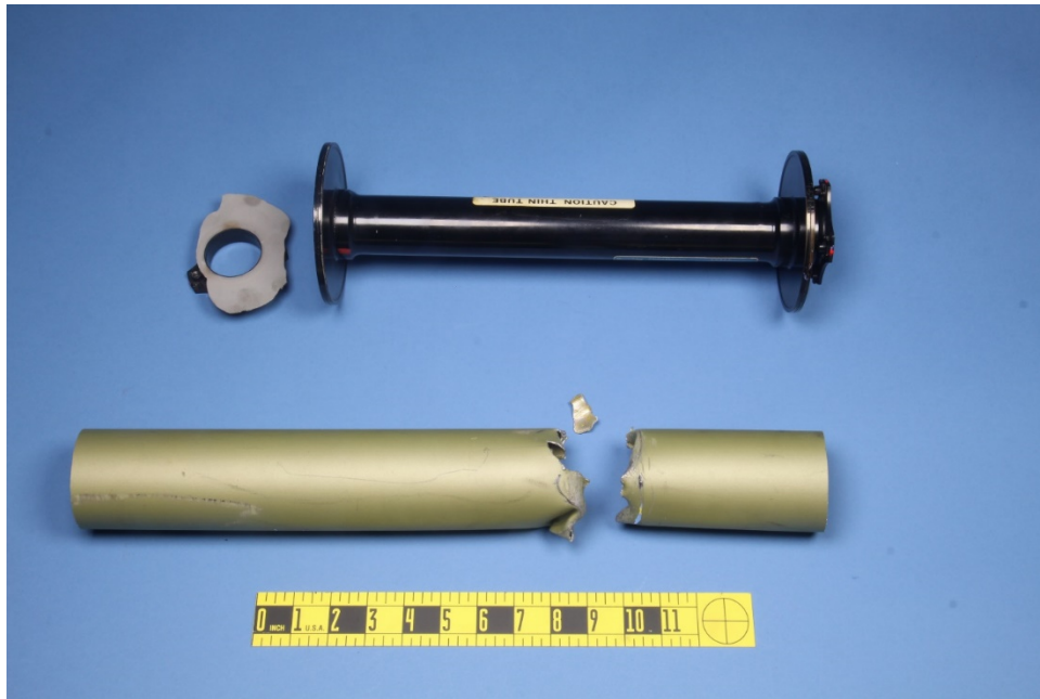
Figure 1: The Main Driveshaft and Section of the Tail Rotor Driveshaft.
