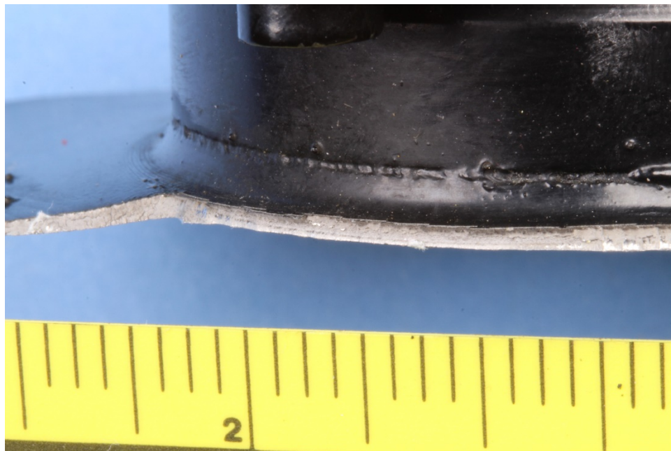
Figure 4: Main Driveshaft Fracture Surface
