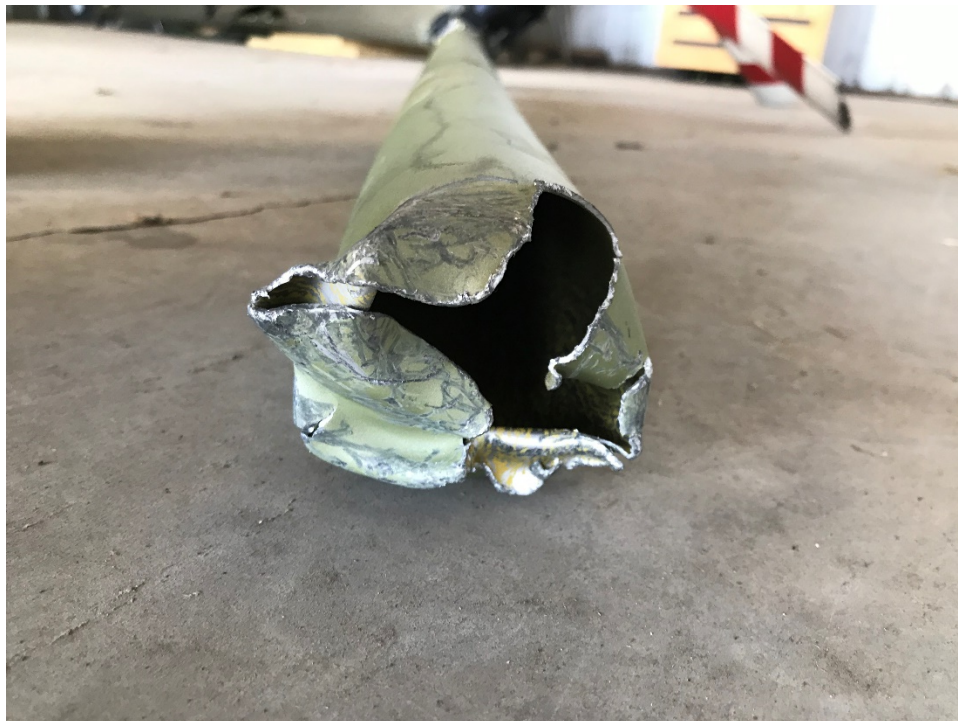
Figure 10: Fracture Surface on Aft Tailboom Driveshaft
