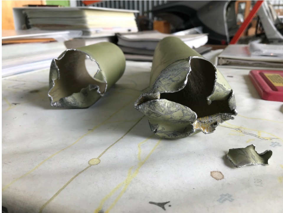
Figure 13: Tailboom Driveshaft Fractures Next to Each Other
