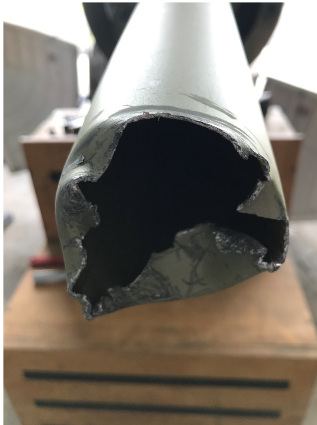
Figure 12: Fracture Surface on Forward Portion of the Tailboom Driveshaft
