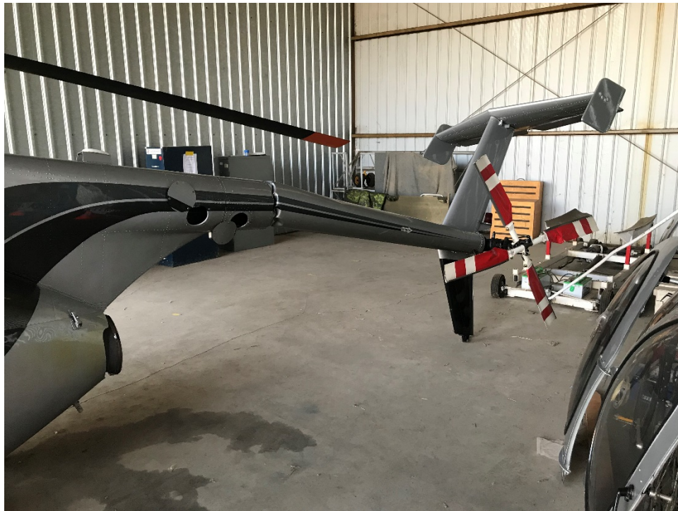
Figure 3: Tailboom and Empennage
