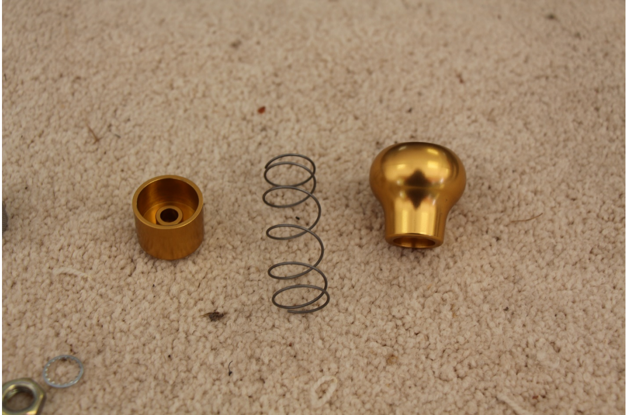
Photograph 3: Throttle Control Assembly Disassembled
