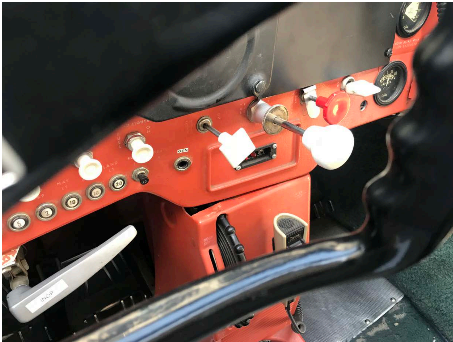
Photo 2 – Carburetor Heat Position After Accident (Courtesy of Federal Aviation Administration)
