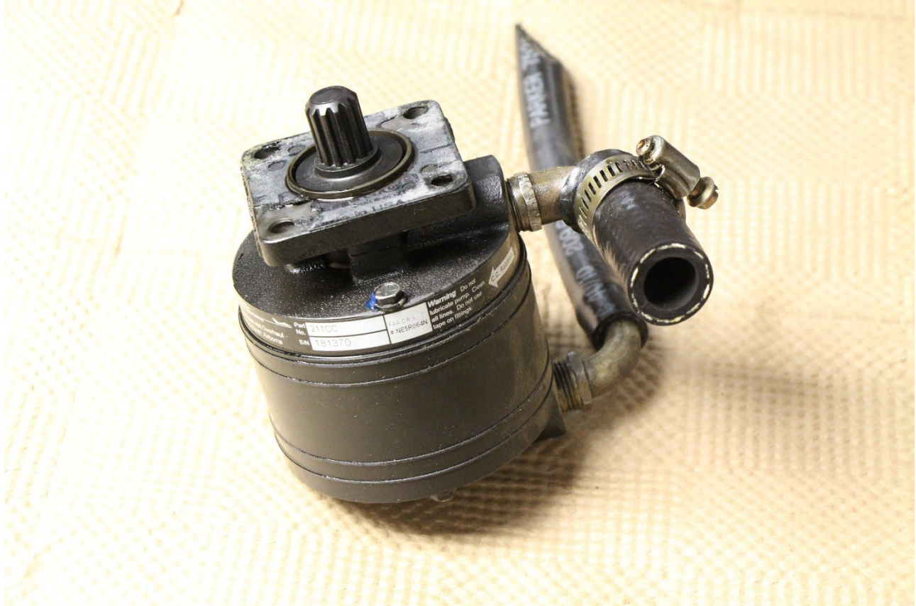
Photograph 7: Right Vacuum Pump
