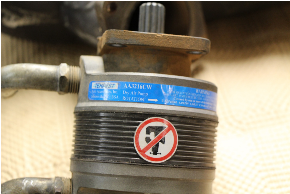
Photograph 8: Left Vacuum Pump
