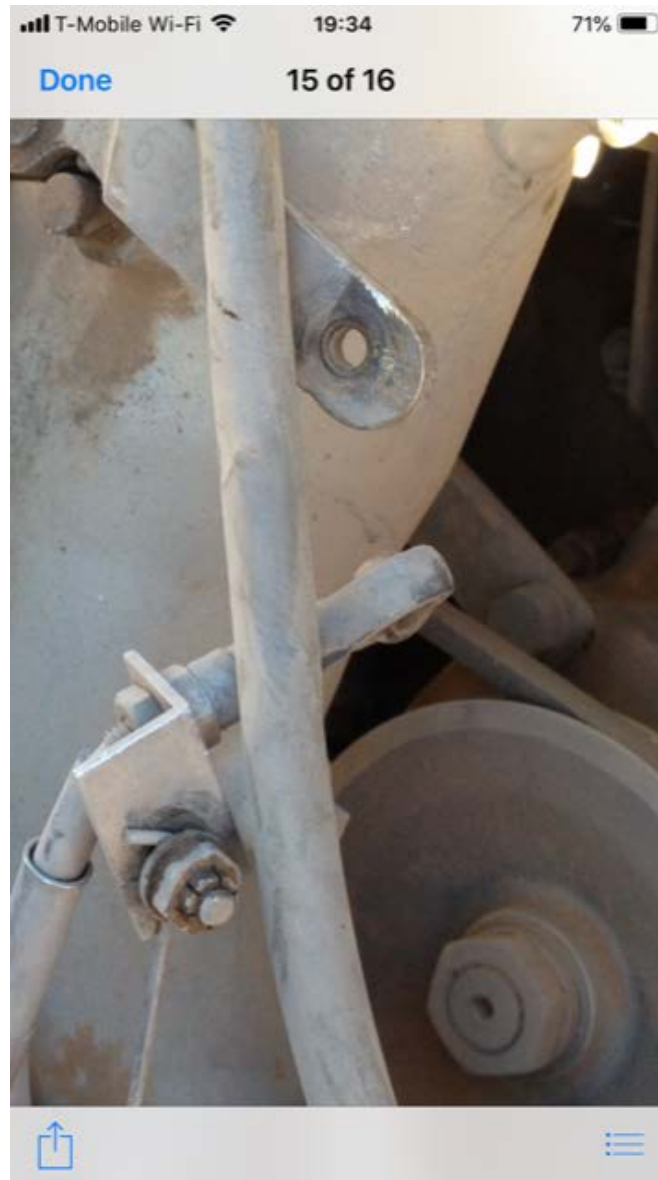
Photo 3 – Throttle Arm Minutes After Accident (Courtesy of Accident Pilot)
