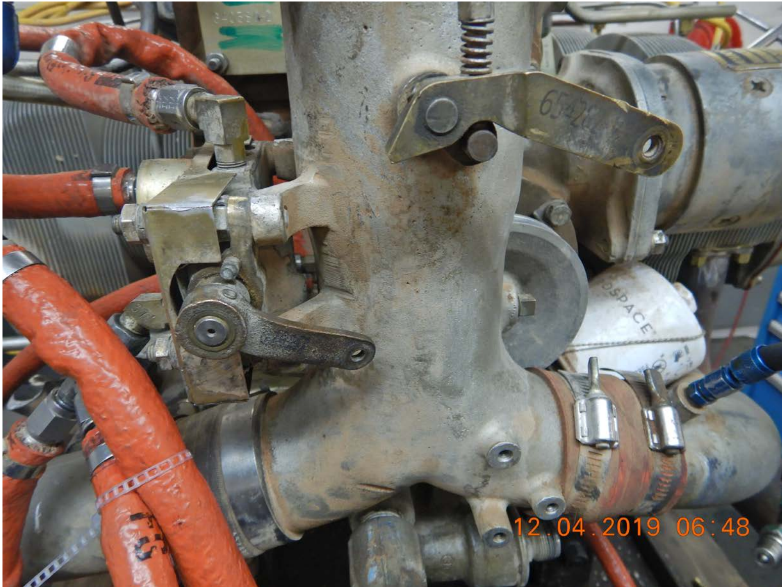
Photo 4 – Mixture Control and Throttle Control Arms (from left to right) (Courtesy of Continental Aerospace Technologies)
