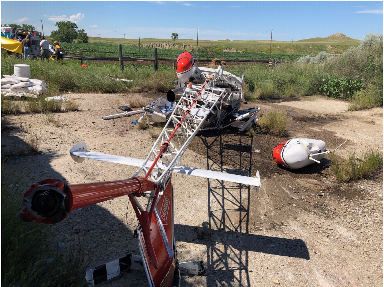
Figure 1. N3078G, rear-view, showing lower section of the 90° gear box. The tail rotor assembly is partially concealed by the vertical stabilizer. Photo courtesy of first responders.
