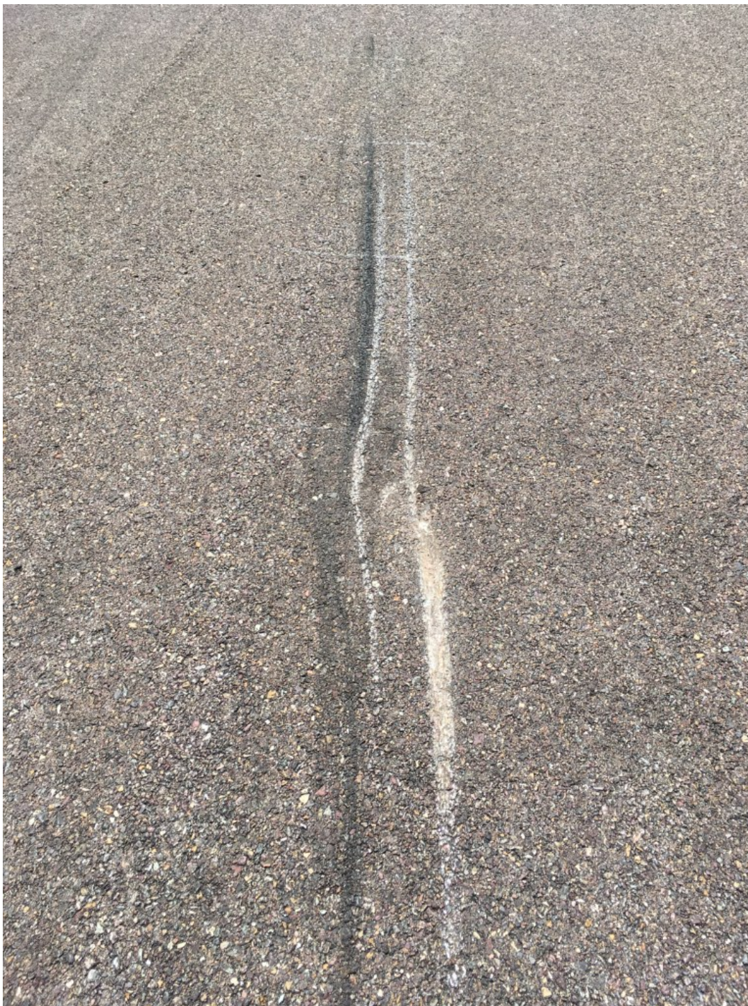
Figure 4 - Second NLG Metal Strike Scar (Note propeller strikes)
