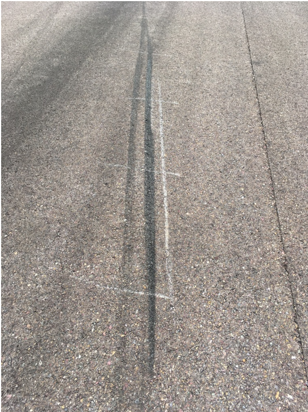
Figure 6 – Third NLG Metal Strike Scar (Note prop strikes)
