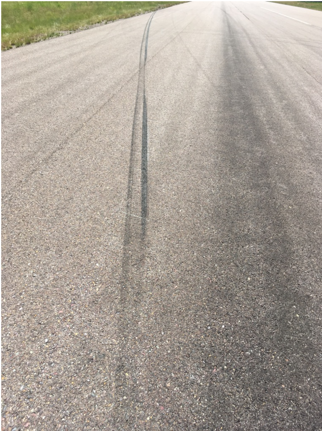
Figure 7 - NLG and RMLG Tire Skid Marks
