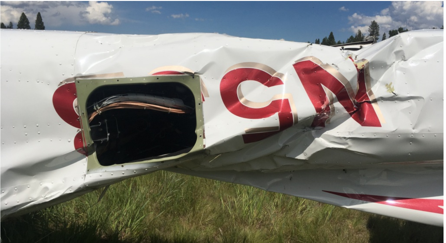
Figure 5 - Aft Right Fuselage (ELT access panel removed)
