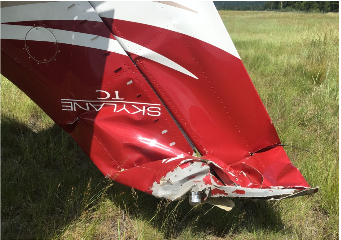
Figure 12 - Vertical Stabilizer and Rudder
