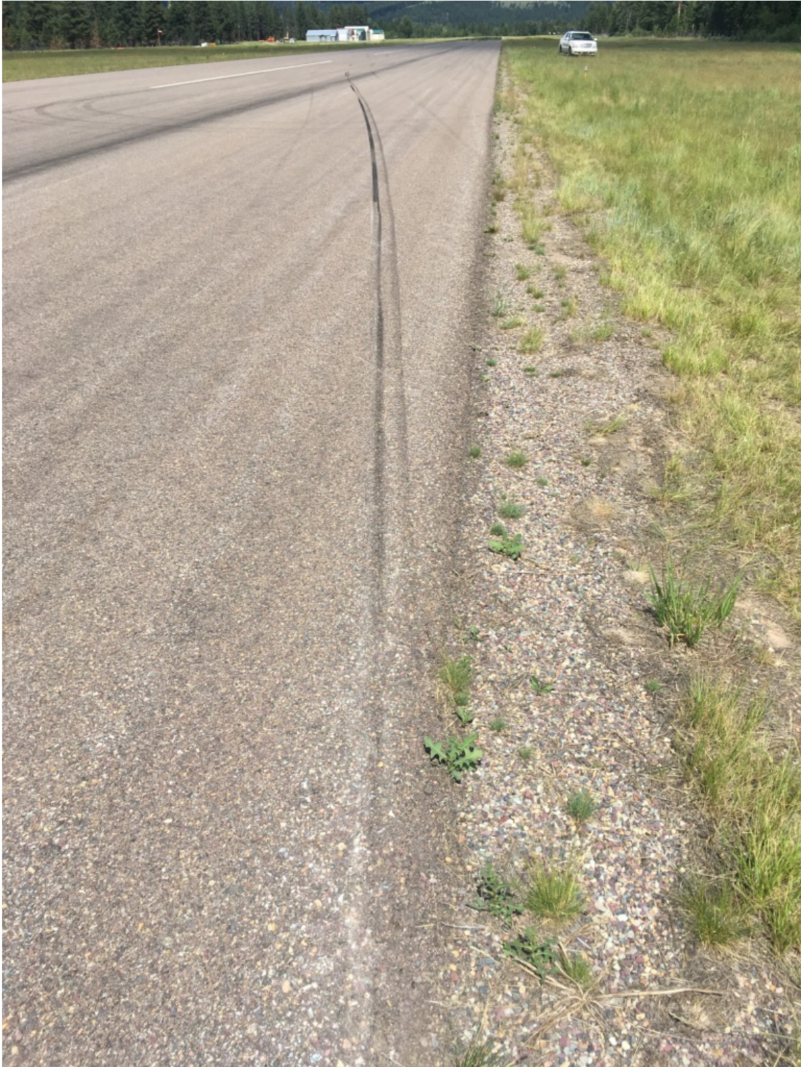
Figure 1 - Skid Mark (view opposite travel direction)
